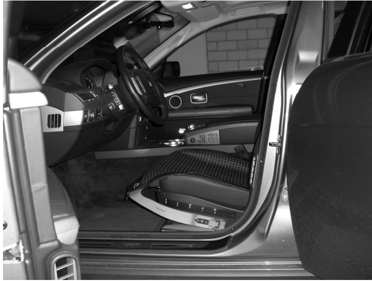
Figure 3.4 Test car with “multifunction seat” and sensormat
