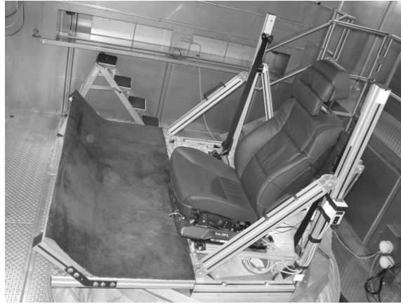
Figure 5.8 Seat with headrest and neck support in the Hexapod
