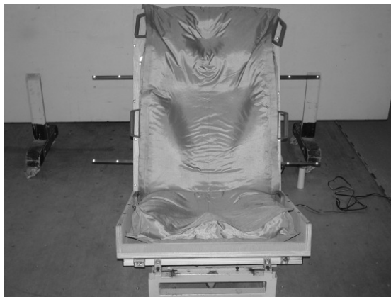
Figure 7.1 Frame with rescue mat after imprinting in the lab
