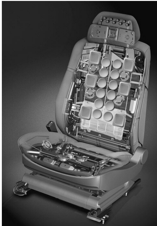
Figure 2.1 Interior of the seat backrest showing the LWMAS, the massage actuators in the middle (round) and the 6 movement actuators in the lateral region (square).
