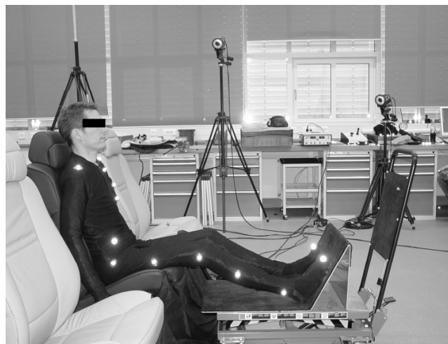
Figure 6.5 Seats with test subject on the sub-frame with footrest in measuring position
