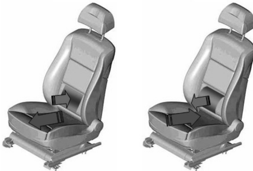
Figure 6.4 Shift function of the new lumbar support
