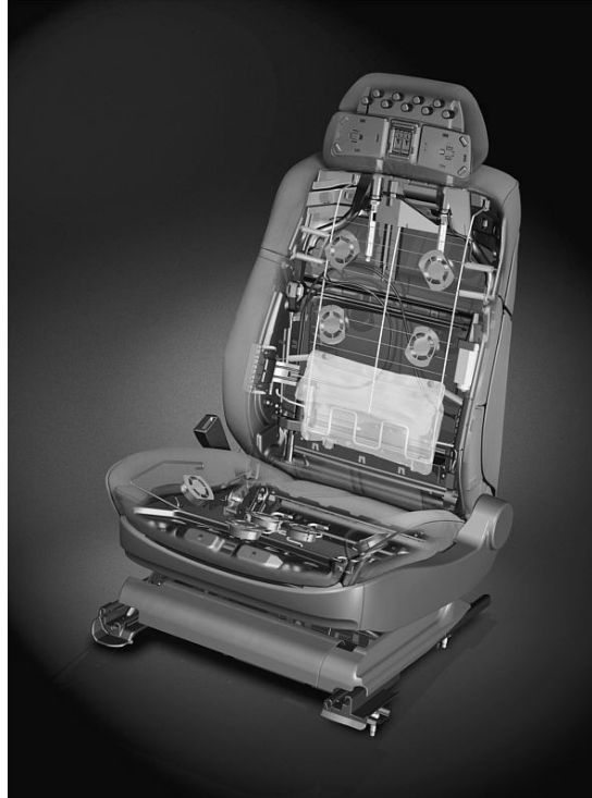
Figure 6.1 Seat with an adjustable standard lumbar support
