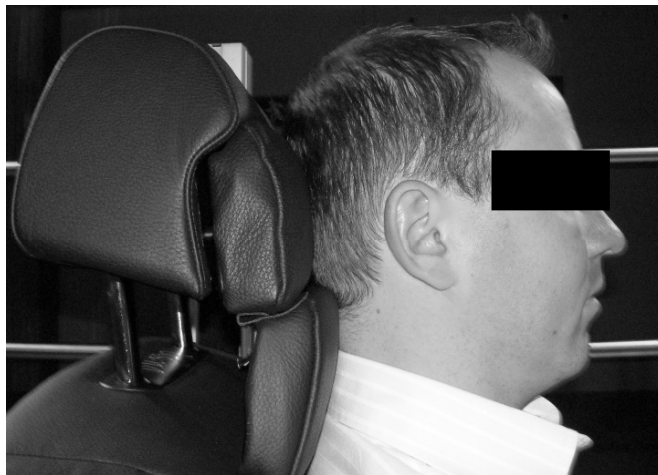
Figure 4.10 Test subject using the headrest with neck support
