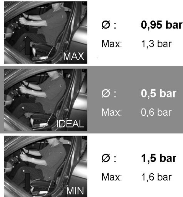
Figure 4.7 Pressure in the disc according to the different seat settings
