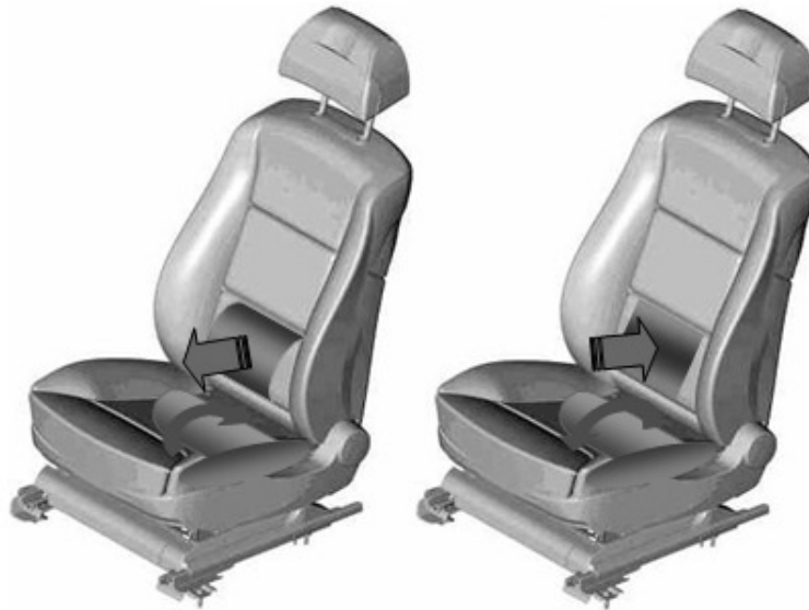
Figure 6.3 Roll function of the new lumbar support
