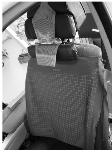
Figure 5.5 Pressure mats used in this study to measure pressure between neck, shoulder and head and seat
