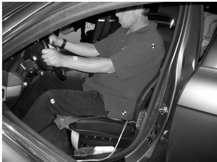
Figure 3.5 Test person with the intradiscal sensor in the car
