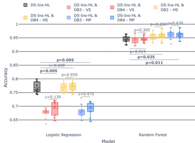
Fig. 48: Validation accuracy score of DS-Ins-HL, DS-Ins-HL with vertical (VS), horizontal stacking (HS), and mean pooling (MP) when using DNABERT with 3-mer and 4-mer (url1). HS and MP features have a dimensionality of 768. VS has a dimensionality of 15 dimensions for each token (DB3=795; DB4=780). Both HS and VS are generated using UMAP as the dimensionality reduction technique. LR and RF models do not report a significant difference among any stacking techniques.
