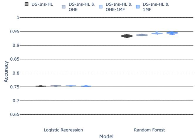
Fig. 41: Test accuracy scores for the DS-Ins-HL feature group and all the encoding techniques. The same trends observed with the train and validation sets persist. 1MF frequency encoding yields the highest accuracy for the RF model, with no difference between performs 1MF and OHE-1MF.
