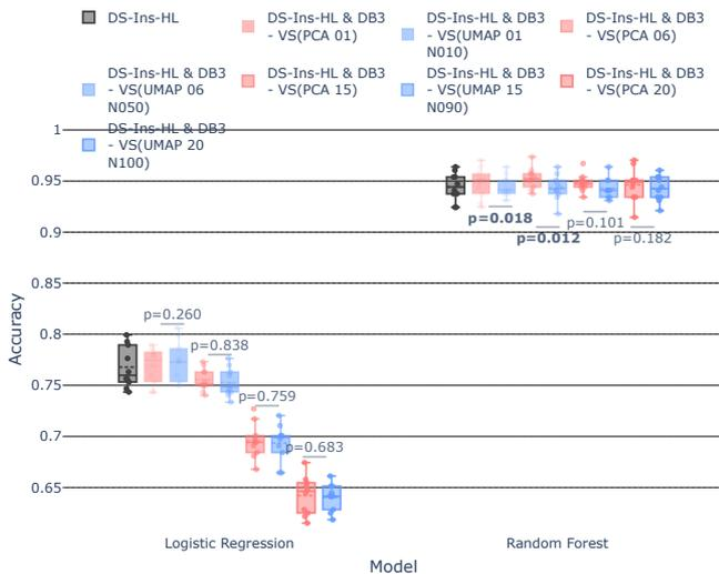
Fig. 45: Validation accuracy score of DS-Ins-HL when using Vertical Stacking (ur1). Those shaded in red are calculated using PCA as a dimensionality reduction, whereas those in blue are calculated using UMAP as a dimensionality reduction technique.
