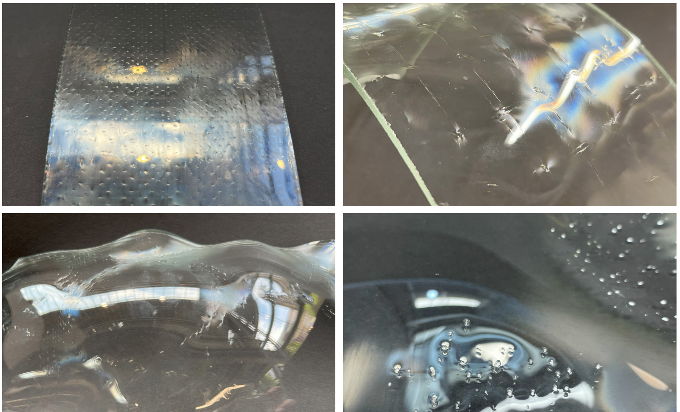
Figure 184: Imprinted texture results. Up left: sample 1.A exhibiting more texture points. Up right: sample 2.B exhibiting stronger texture almost revealing the whole mould shape. Down left: Texture from changing mould support by change of pattern resulting to texture only at the edge of the change. Down right: texture of sample 9 showing strong texture only from the cement coating and not from the textile. Own images.
