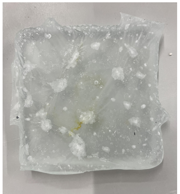
Figure 175: Intensified stress test 2: glass-basalt cast tile. Before (left) and (after) casting. Source: Left: T.Bristogianni, Right: own image.
