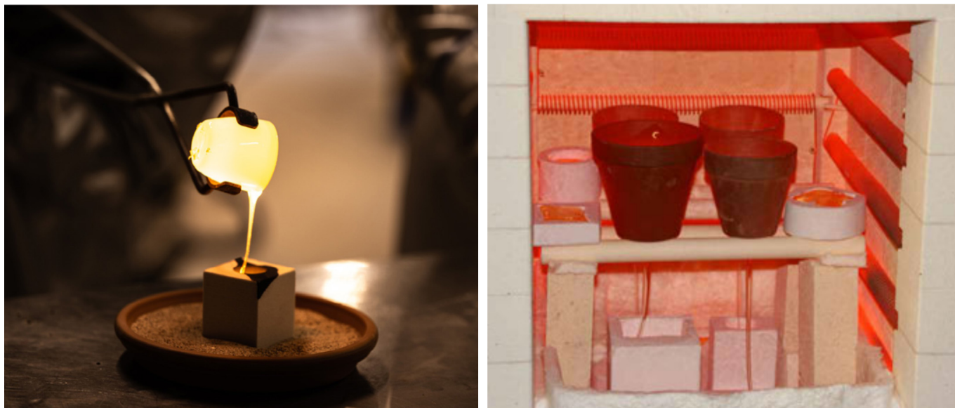
Figure 29: Glass casting: primary (left) and secondary (right) casting process. Source: left: Marcel Bilow, right: Oikonomopoulou, 2019.
