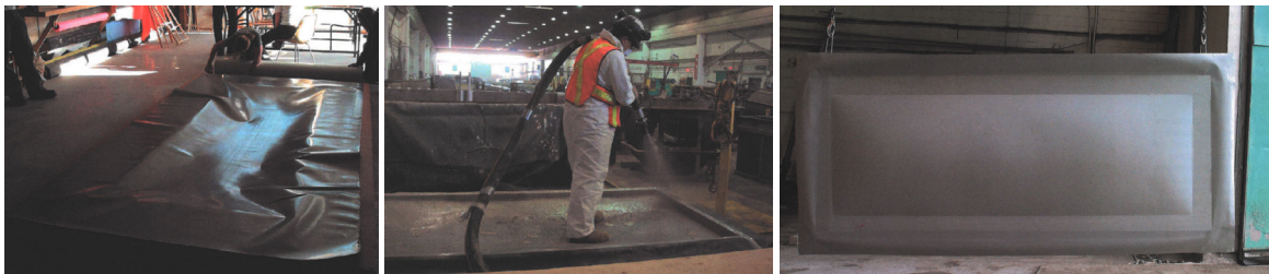
Figure 73: Horizontal hanging mould. Source: West, 2016.
