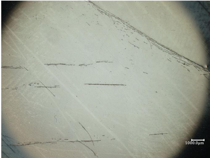
Figure 169: Sample 6 under the microscope: basalt fiber inclusions and stretch marks on opposite glass surface. Own images.
