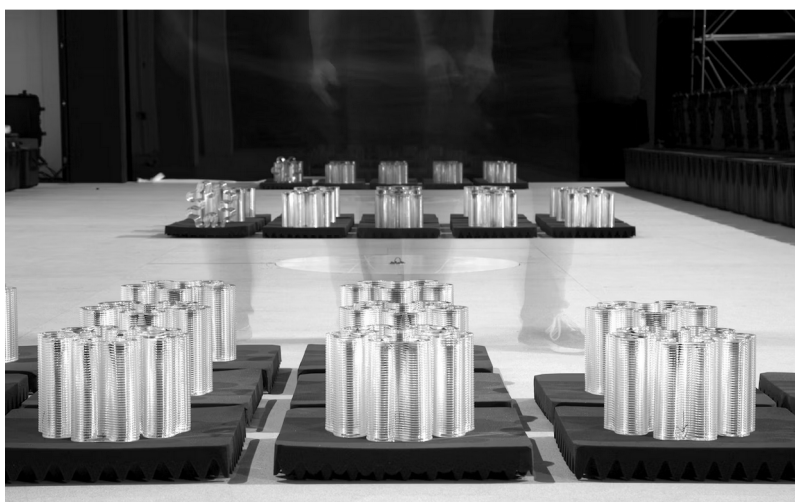
Figure 49: Glass II - 3d printed glass column. Down: disassembled. Source: www.oxman.com.
