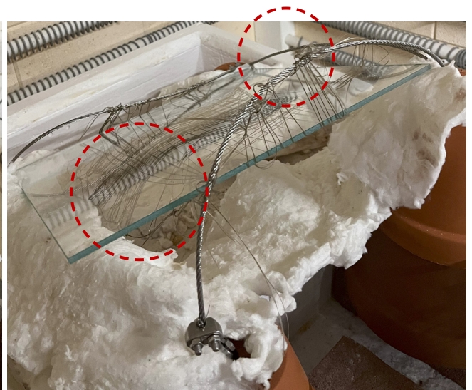
Figure 138: Left: Set-up of experiment 6 in the oven. Right: placement of glass on mould and failure locations (circles). Own image.
