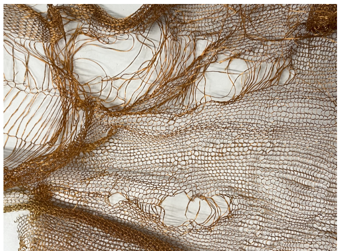
Figure 147: Unraveled and broken mould 7.A after the slumping process. Own image.
