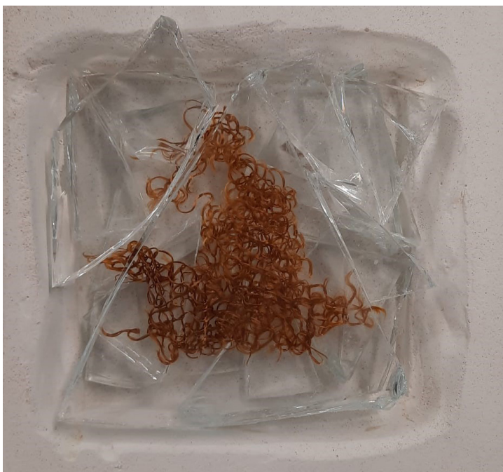
Figure 175: Intensified stress test 2: glass-basalt cast tile. Before (left) and (after) casting. Source: Left: T.Bristogianni, Right: own image.
