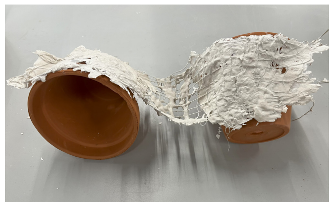
Figure 132: Hand-woven mould dipped in Crystalcast plaster and stabilized in place. Own image.
