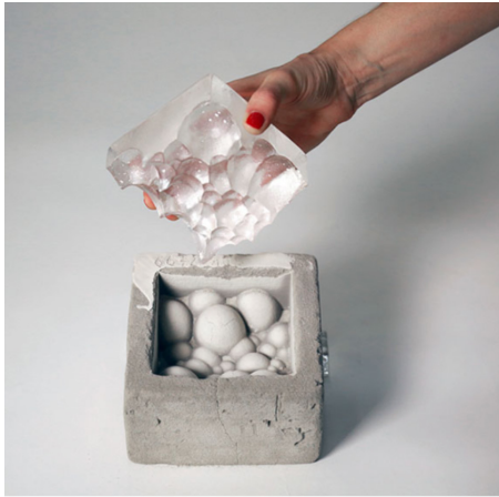
Figure 3: 3d printed sand mould for glass casting. Source: Giesecke & Dillenburger, 2022.
