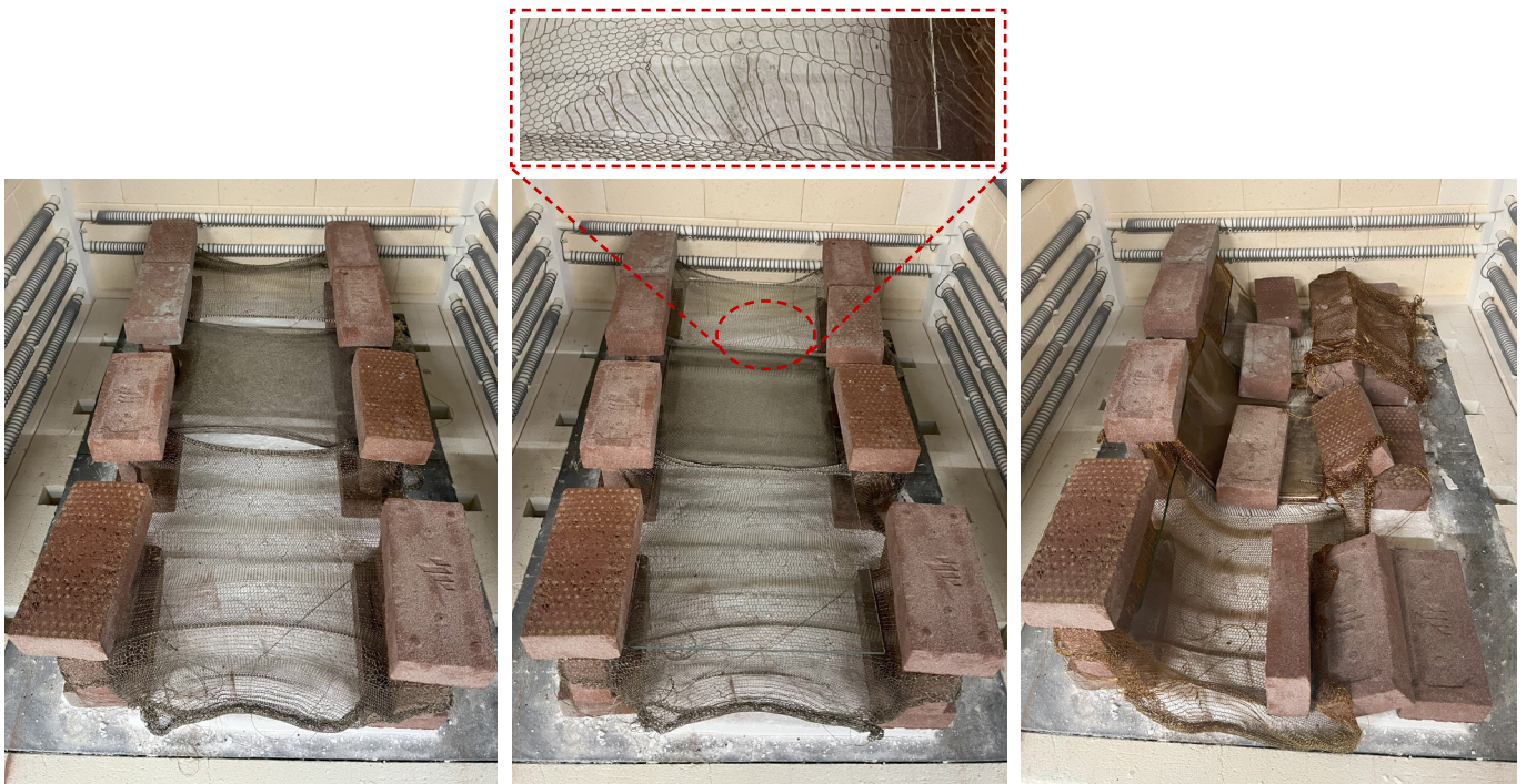
Figure 144: Experiment 7 set-up in the oven. Left: placement of moulds, Middle: with glass pieces on top and beginning of unraveling of 7.A, Right: after slumping process. Own images.
