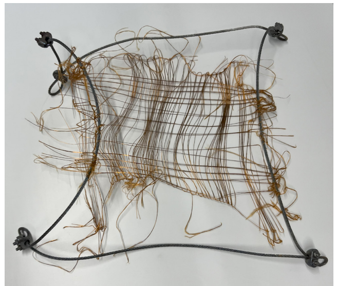
Figure 140: Mould after the slumping process. Own image.
