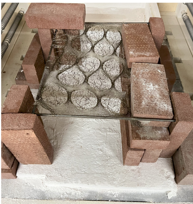
Figure 152: Experiment 8 set-up in the oven. Left: placement of mould, Right: after slumping process. Own images.
