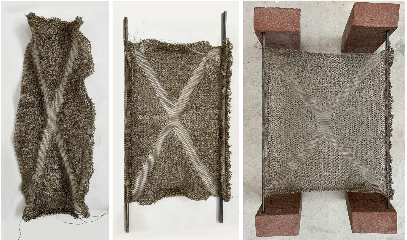
Figure 189: Basalt knitted mould; relaxed (left), with bars in the cannel (middle) and tensioned (right). Own images.
