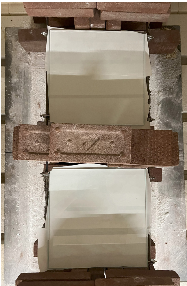
Figure 192: Set-up of prototype in the oven. Up right: mould set up: above sample B and down sample A. Down left: before slumping. Down right: After slumping. Own images.
