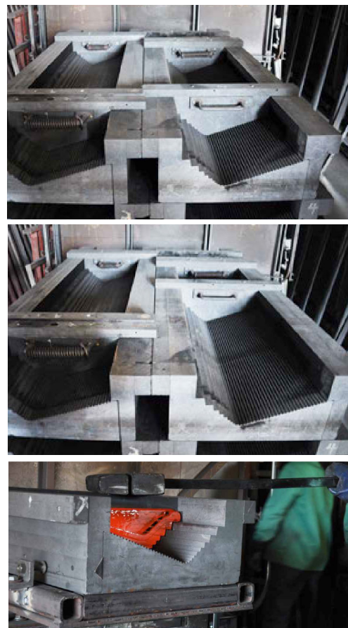
Figure 56: Adjustable graphite mould at John Lewis Glass Studio for the components of the Ice Falls project by James Carpenter. Source: Oikonomopoulou, 2019.
