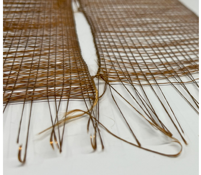
Figure 111: Breakage of supports of mould. Own image.
