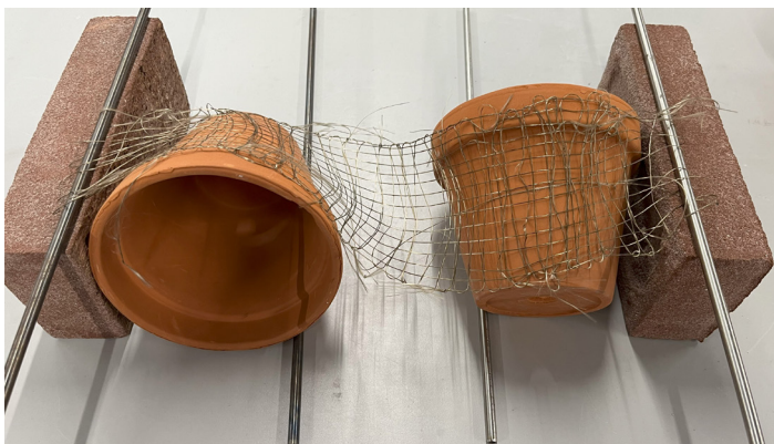
Figure 131: Setup of geometry with hand-woven loose weave mould. Own image.
