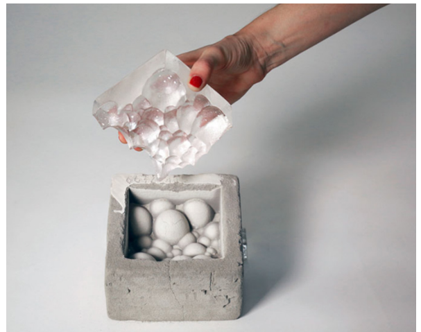
Figure 53: Disposable mould out of plaster and silica sand. Source: Oikonomopoulou, 2019.
