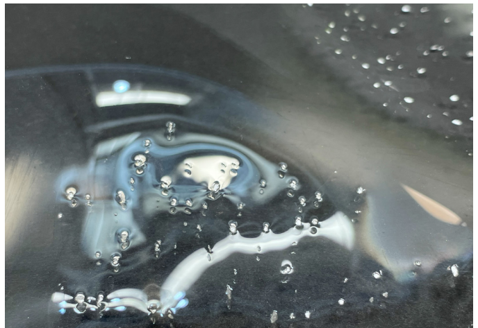
Figure 162: Glass texture: inclusions of cement - dot like texture. Own image.
