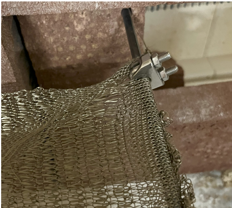
Figure 190: Clamps for maintaining the tensioned mould shape in a controlled position. Own image.
