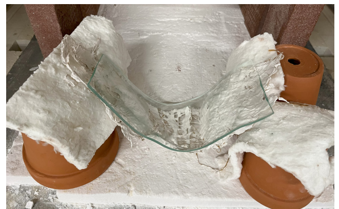
Figure 133: Set-up of experiment 5 in the oven. Before (left) and after (right) slumping. Own image.
