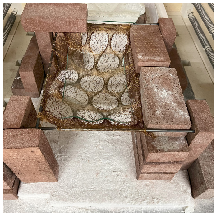
Figure 152: Experiment 8 set-up in the oven. Left: placement of mould, Right: after slumping process. Own images.
