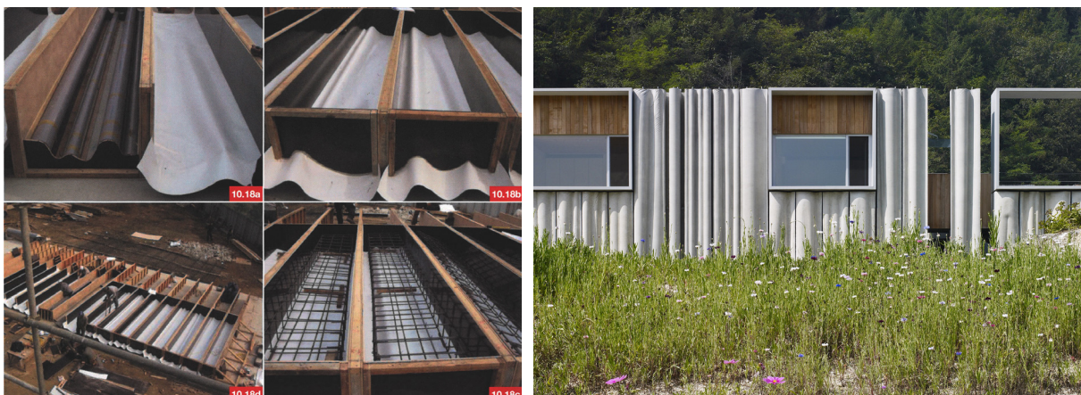
Figure 72: Left: Open through mould. Source: West, 2016. Right: Hanil Company Visitors Center façade. Source: www.archdaily.com
