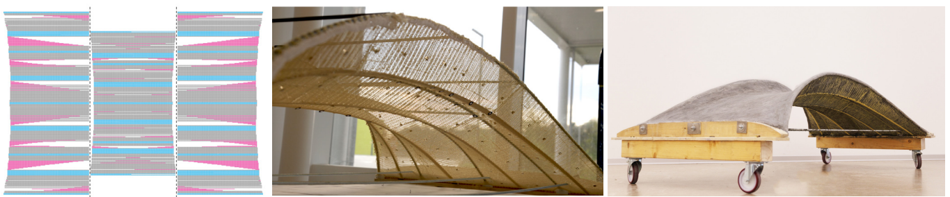
Figure 79: knitCrete Bridge. Left: knitting pattern, Middle: mould tensioned in place. Source: Popescu, 2019. Right: prototype. Source: www.block.arch.ethz.ch.
