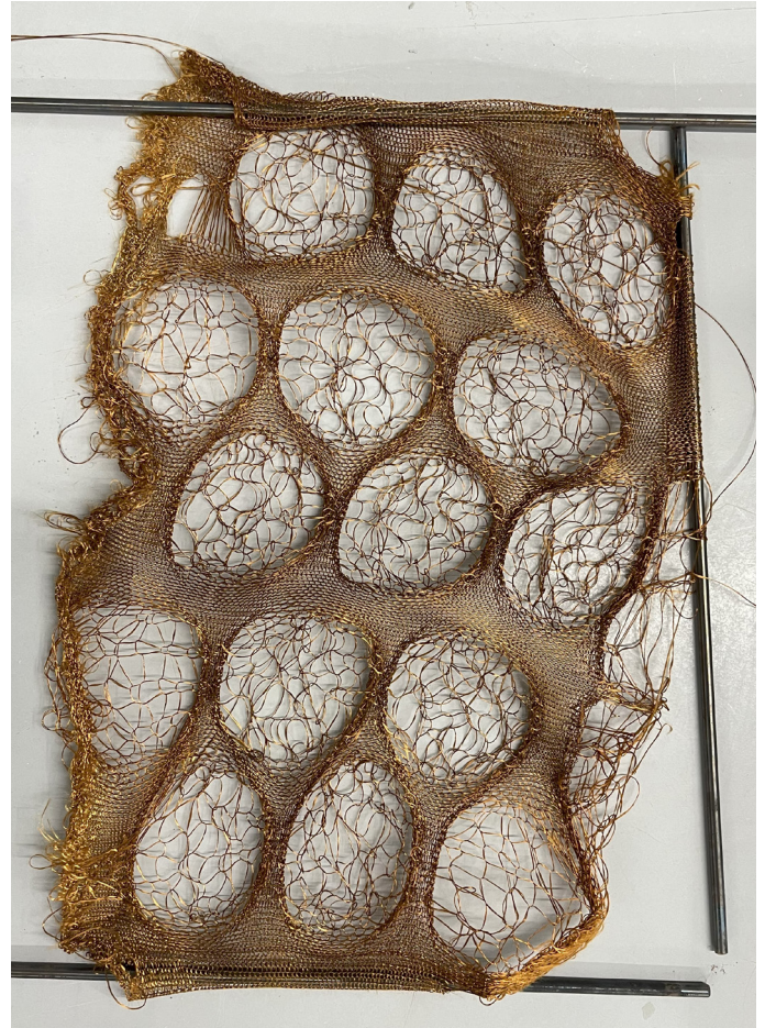
Figure 153: Bubble knit mould after the slumping process. Own image.
