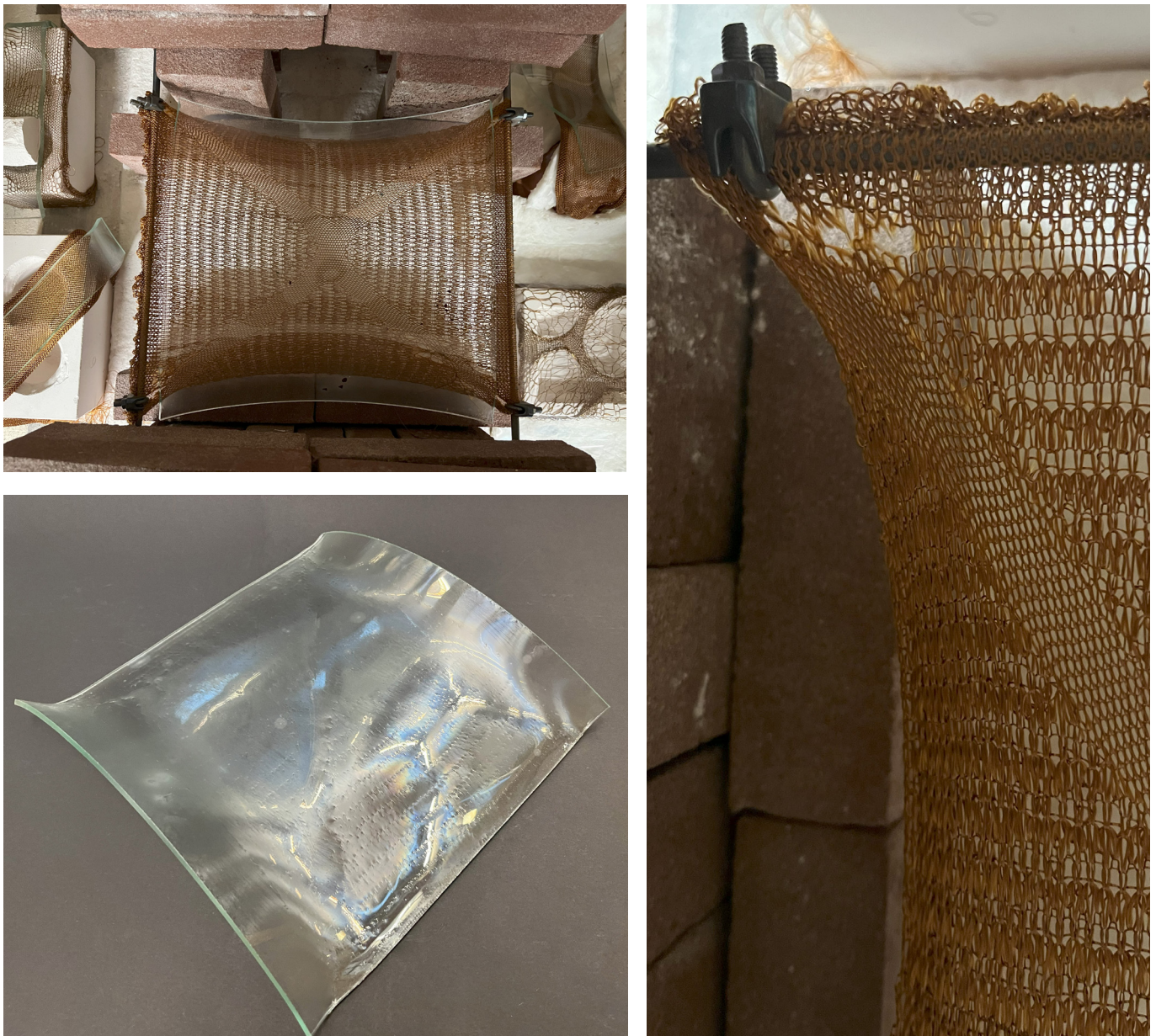
Figure 200: Left top: Mould reuse with single piece of glass after slumping. Left bottom: resulting glass geometry similar to 1st time use of mould. Right: Mould teared and stretched after 2nd slumping process. Own images.
