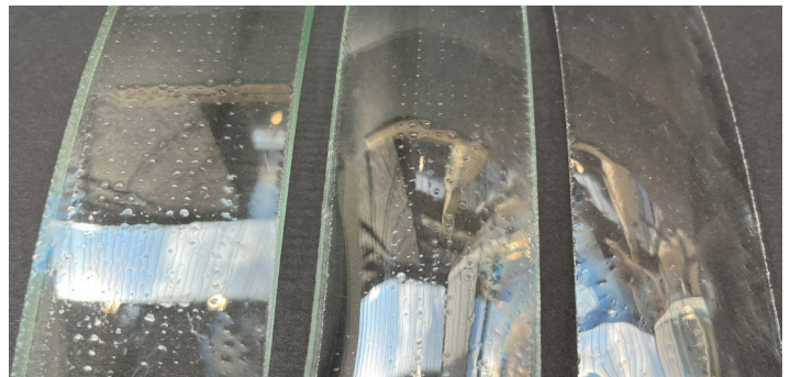
Figure 127: Resulting surface of glasses of 4.A, 4.B, 4.D (left to right); 4.B with coating results in slightly better surface than the others. Own image.
