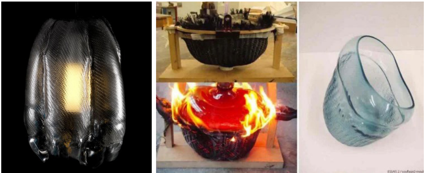
Figure 26: Left: Textured vase by Claire Baudrimont. Source: www.ecal.ch . Right: Process of texturing the glass with carbon fiber mould. Source: www.art-folio.ch .
