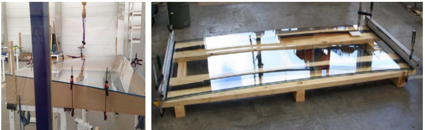
Figure 58: Left: Cold bending on final frame. Source: Glass Performance Days ( www.gpd.fj ). Right: Cold bending by lamination. Source: McDonnell et al., 2018.
