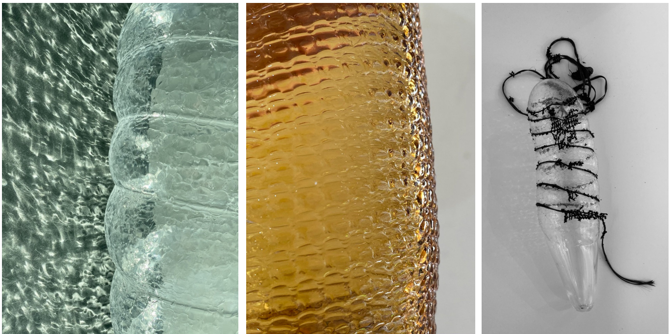
Figure 27: Left & Middle: Textured object with knitted mould by Mariana Popescu. Right: Glass blown object with the remaining of the knit textile mould. Source: www.maadpope.com .
