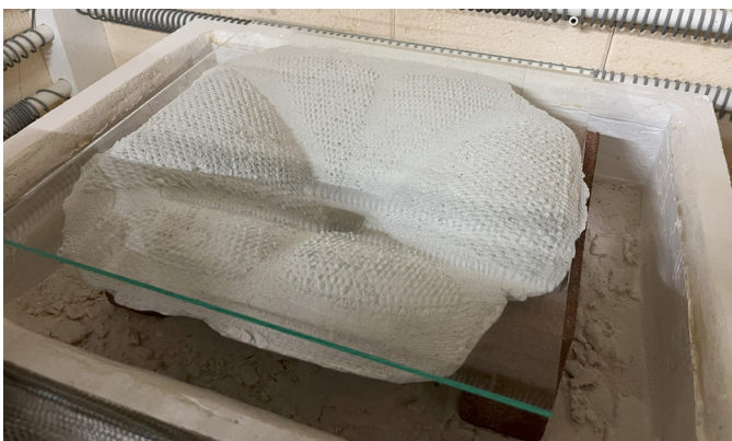
Figure 160: Experiment 9 set-up in the oven before (left) and after (right) slumping. Own images.
