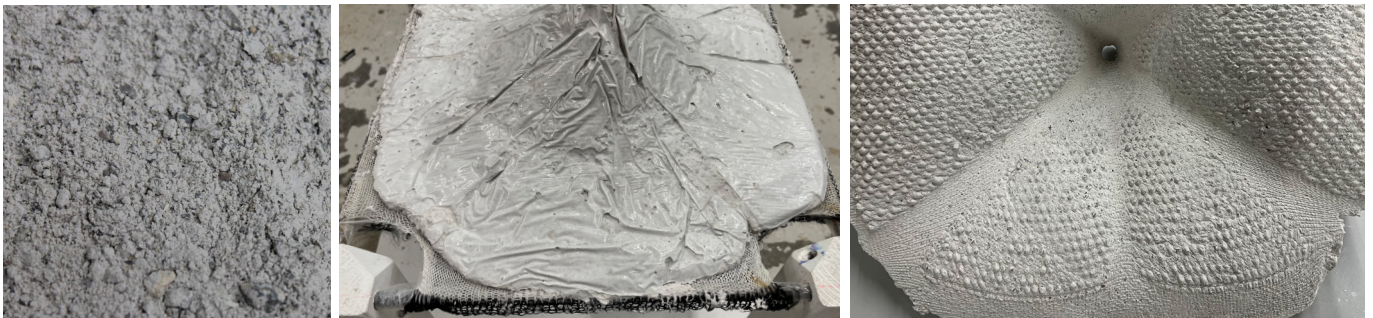
Figure 97: Left: Heat resistant cement mix. Source: www.glsmbh.de . Middle & Right: Heat resistant cement used on textile formwork for sample preparation: cement on textile (middle) and result (right). Geometry & formwork developed by Kariouh and Popescu [2024]. Own images.
