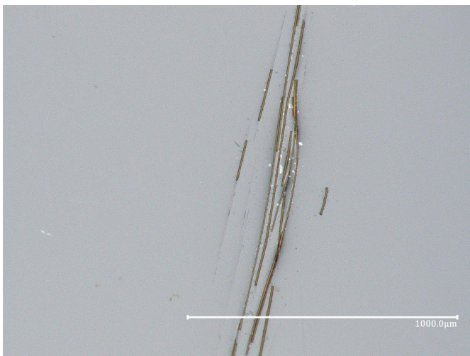
Figure 165: Sample 1B under the microscope. Up: basalt inclusions - left: pattern - right: with polarization filter. Down: Zoomed in images of basalt fibers inclusion with normal (left) and polarization filter (right). Own images.
