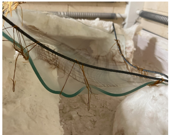
Figure 139: Experiment 6 in the oven, results after slumping. Own images.
