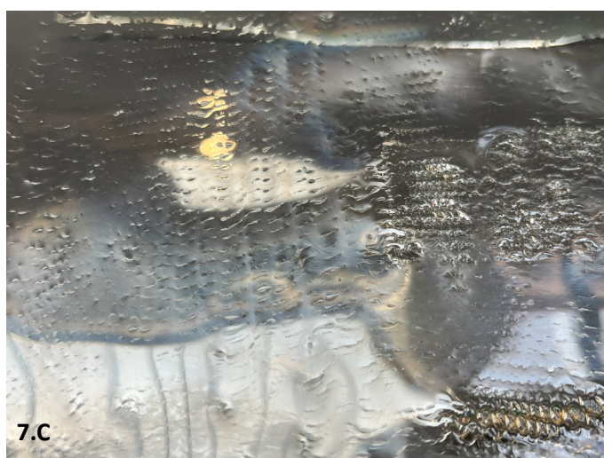
Figure 149: Imprinted texture from moulds. Own images.
