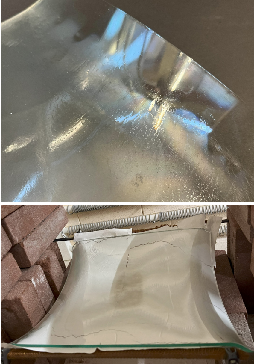
Figure 202: Up: Finishing surface of 4mm glasses. Down: Thin fire paper wrinkles and shreds resulting in glass texture. Own images.
