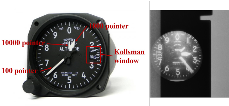
Figure 3.8: Example for a physical altimeter and its equivalent from a historical image of the TMA archive. Adapted from UK Airports (2022).
