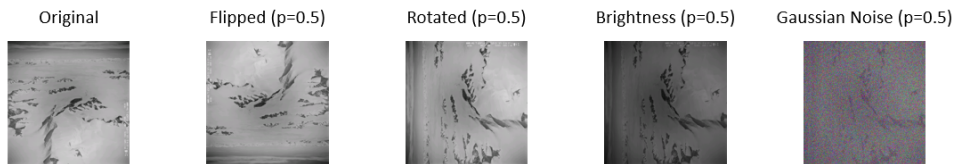
Figure 2.7: Four different augmentation methods of the training images together with their probability.
