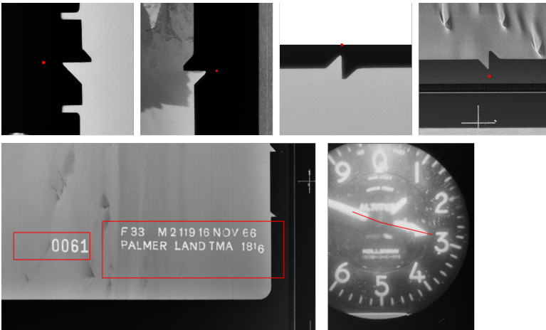
Figure 3.10: Examples for successful detections: Fiducial marks (top), text extraction (bottom left) and altitude based on altimeter (bottom right)
