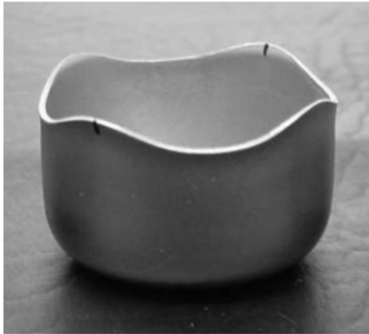
Figure 1.1: Undesirable 'Earrings' formed during deep drawing processes
