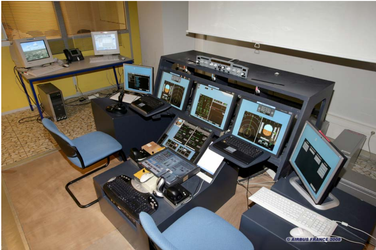
Figure 7-21: the research simulator is used for early prototyping of HMI design
