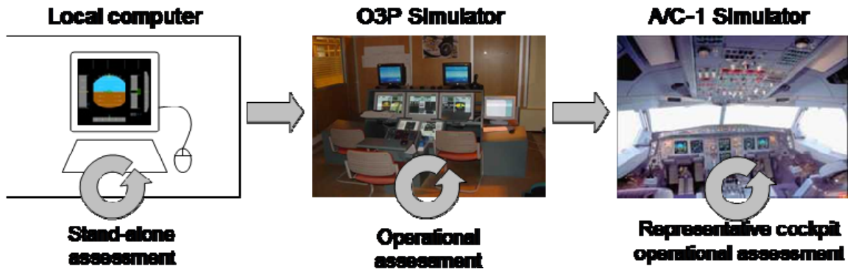
Figure 7-1: A full design procedure in sets of iterations on three increasing representative simulators.
