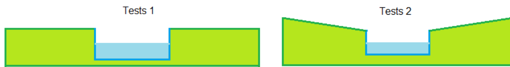
Figure 5-8 Cross section of the area with no slope and a small slope in the direction perpendicular to the channel flow
