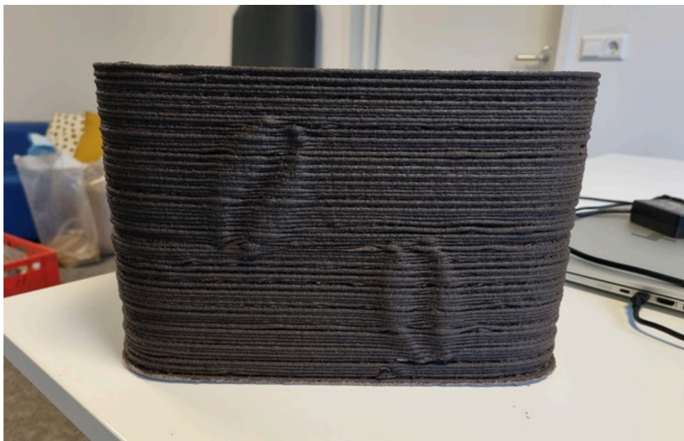
Figure 35: Added texture in the walls of a print
