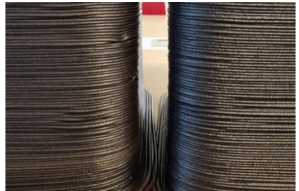
Figure 15: Inconsistency in granulate mix (colour difference)
