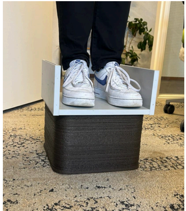
Figure 36: Person standing on square 3D print (bioHDPE)
