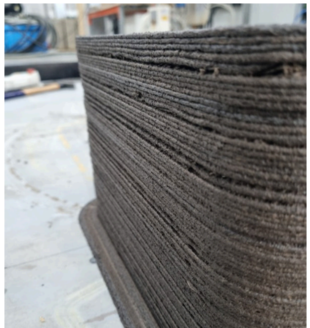
Figure 33: Inconsistent layers (TPS)
