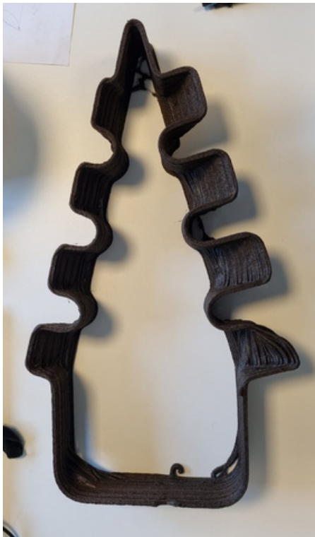
Figure 24: Print samples overhang model
