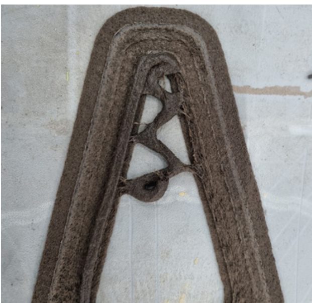
Figure 27: Bridging attempt within the overhang model
