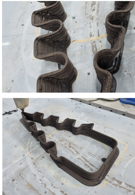
Figure 25: Successful overhang angle (left), failed overhang angle (right)
