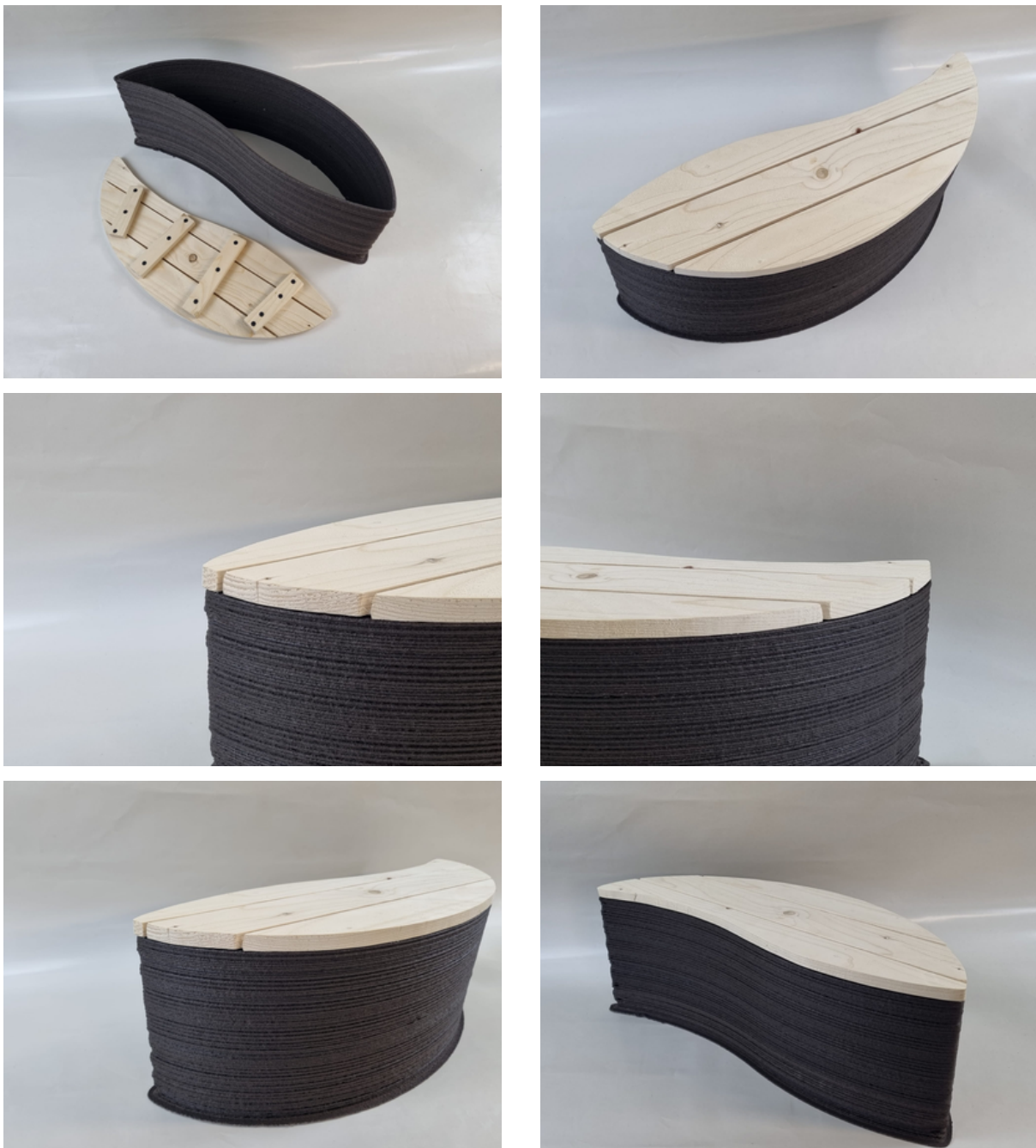
Figure 61: 3D printed prototype on small extruder with wood seat
