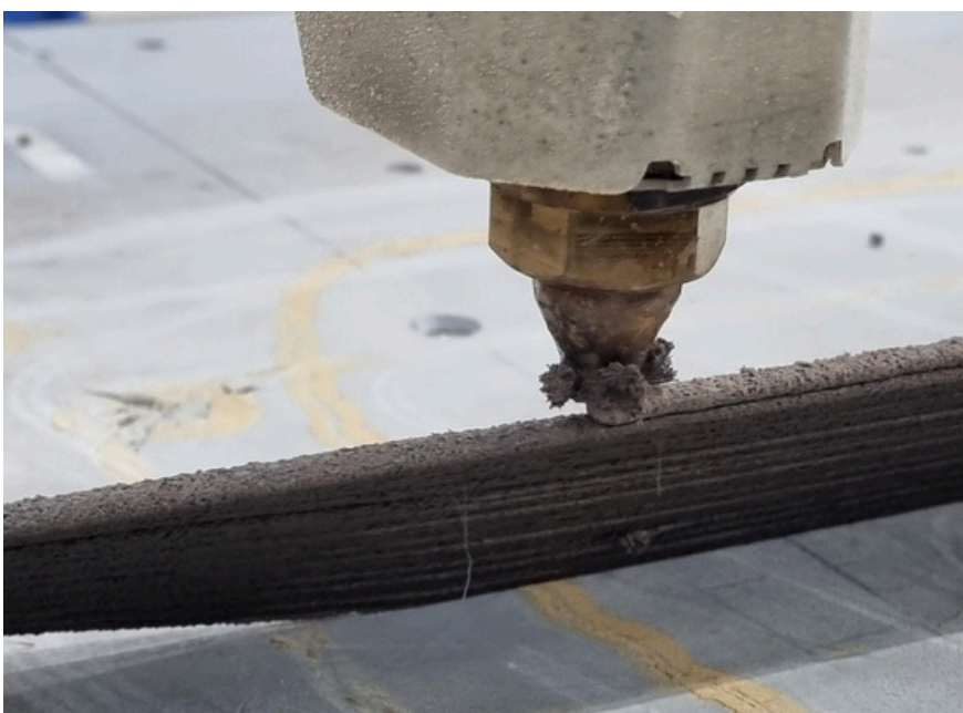
Figure 12: Clogging of the print nozzle
