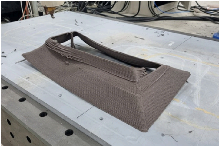
Figure 16: Sagging of the printed walls, rPP (left) and bioHDPE (right)
