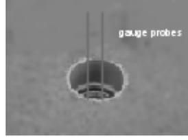
Figure 3. On-crest accommodation well for the overtopping gauge.
