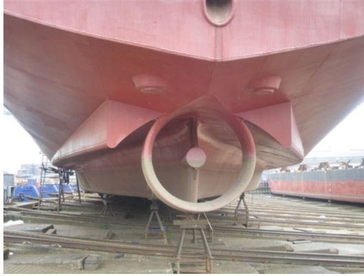
Figure 5.15: An inland ship with a transom and backward-facing tunnel endings (Rotteveel, 2019)
