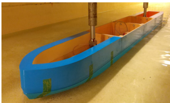
Figure 3.1: The 1/30 scaled model of an inland ship in towing tank
