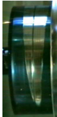
Figure 5.1: Cavitation in a journal bearing [13]. A clear difference can be seen where the oil film has cavitated (the metal surface of the shaft can be seen) and where the oil film is still intact.
