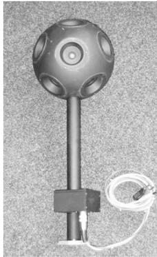
**Figure 4.3:** The Plenopter, a light measuring device capable of capturing local light fields up to the second order. 12 photocells with wide apertures of  $74^\circ$  cover the entire sphere capturing light from all directions.
