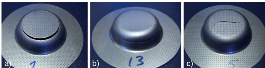
Fig. 7 Different failure modes in the Marciniak test investigated on IF steel (for r_p = 50 mm, r_{pe} = 10 mm): (a) washer hole initiated failure (washer hole too large) (b) deep drawing failure (i.e. the reverse friction effect not sufficiently strong) and (c) successful failure triggering a random crack in the center region
