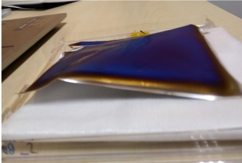
Figure 36: First Substrate/TCO/p-i-n cell deposited in superstrate form on Al foil substrate.
