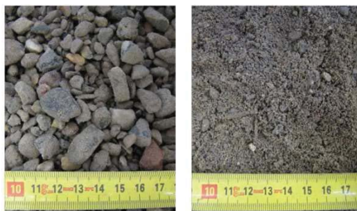
Figure 5. Products from crushed concrete by ADR: Coarse (left) and Fine (right).
