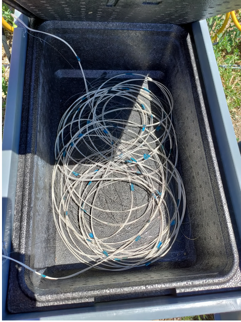
(a) Top view with several fibers, without water, sensors, and mixing equipment
