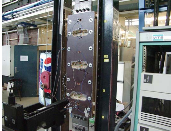
Figure 4.4: Specimen with anti-buckling guides positioned on the fatigue testing machine.
