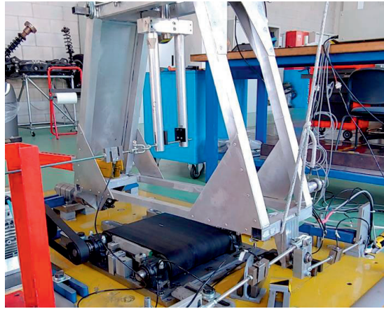
Figure 3.29 – Set-up for the verification of lateral force.
