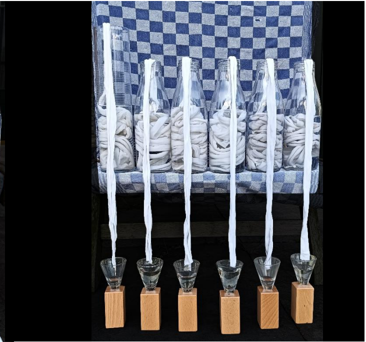
Fig. 42 - Drip test experimentation - drip rate determination
