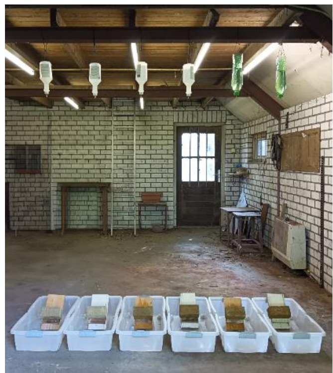
Fig. 39 - Drip test set-up
