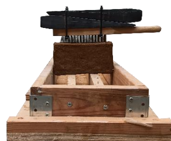
Fig. 30 - Abrasion test set-up
