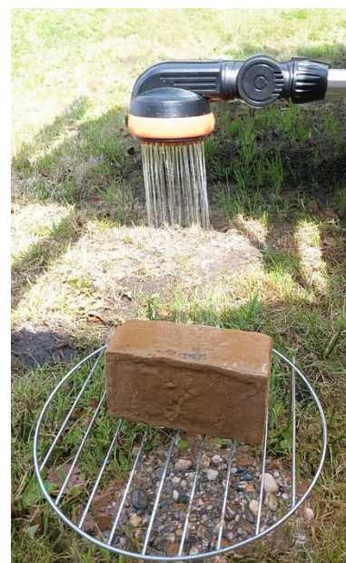
Fig. 45 - Spray test set-up
