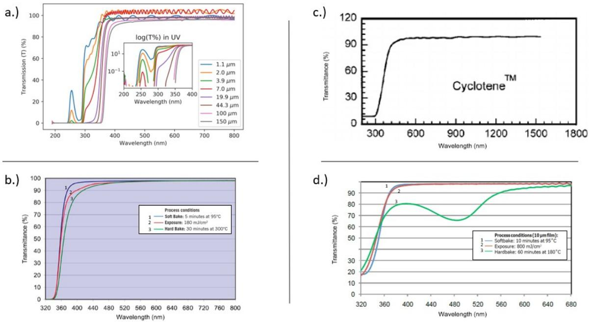
**Figure 5.9:** Overview of graphs on absorption and transmission of the polymers a.) SU-8 thickness [27] b.) SU-8 supplier [4], c.) BCB [28] and d.) permindex [7]
