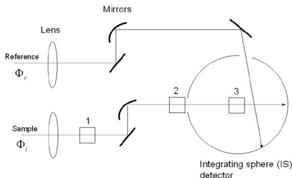
**Figure 5.16:** Schematic light emitted and following two paths at the same time. One bundle being the reference and the other the sample [33].
