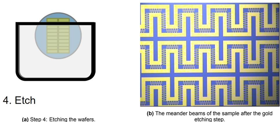
Figure 4.7: Microscopic inspection on the gold wafer structure.
