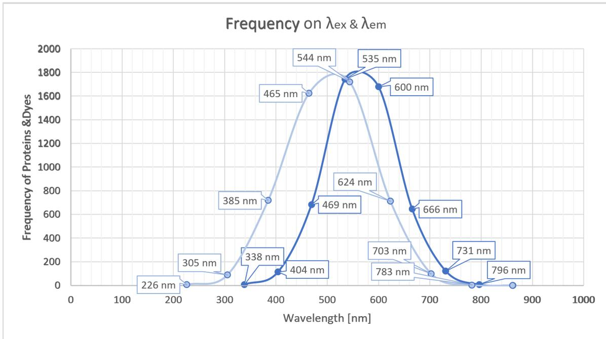
**Figure 5.1:** Distribution of the number of fluorescent dyes and proteins over the wavelength. The light coloured line represents the excitation wavelength and the other represents the emission wavelength.
