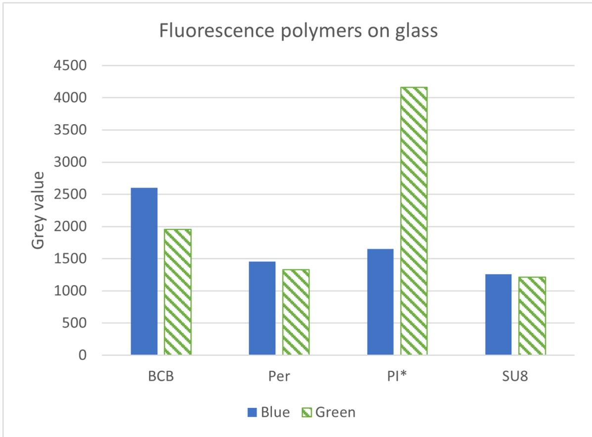
(a) Fluorescence of polymers on glass wafers. Polyimide on a BF33 glass wafer, the others on AF45 glass wafers.
