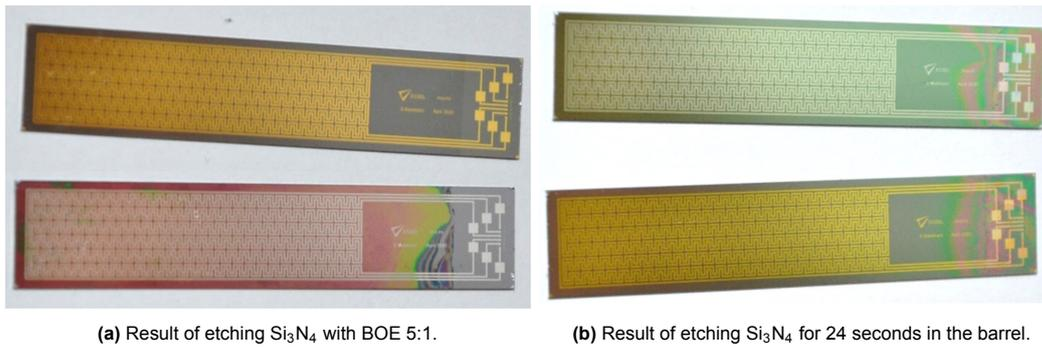
**Figure 7.6:** Silicon Nitride etching of BOE compared to barrel.
