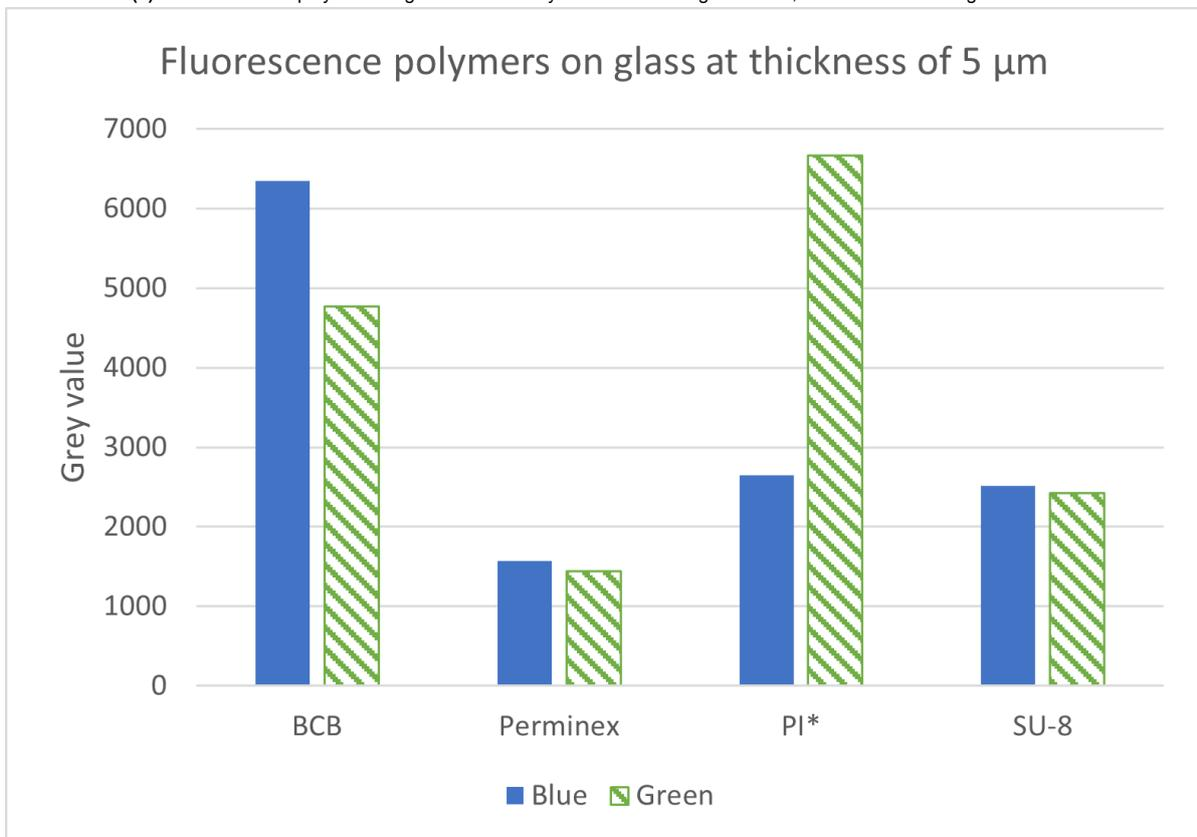
(b) Fluorescence of polymers with normalization to 5 micrometers
