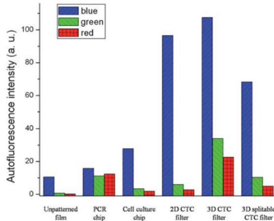
**Figure 5.5:** Fluorescent intensity of parylene-C per device sample [20].
