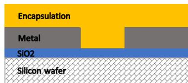
**Figure 4.2:** Structural layers of hermeticity samples.
