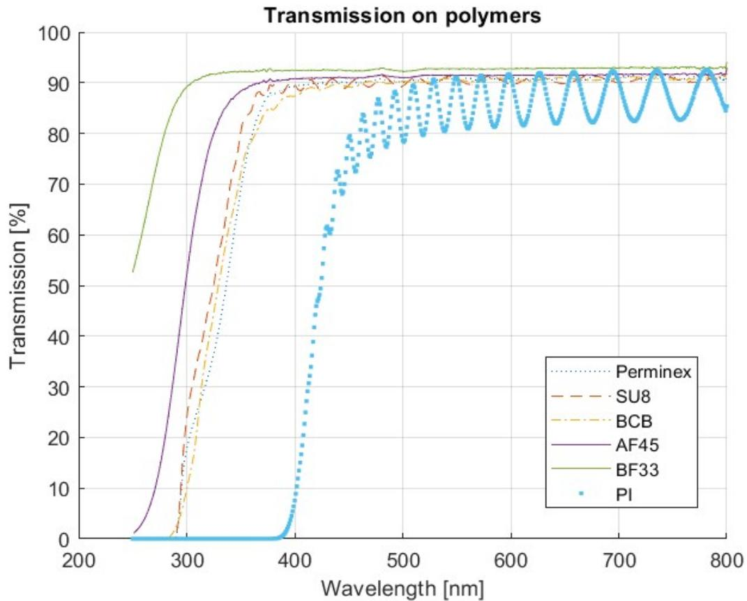
Figure 5.23: Transmission of polymers
