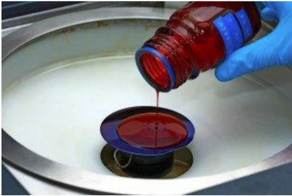
**Figure 4.1:** An illustration of how a polymer can be applied when a wafer is on a spin coater [15].
