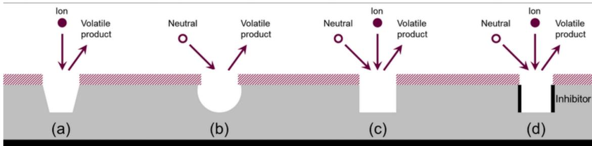
14: Description of basic etching processes: (a) sputtering, (b) pure chemical etching, (c) ion-assisted etching, and (d) ion-enhanced inhibitor etching.
