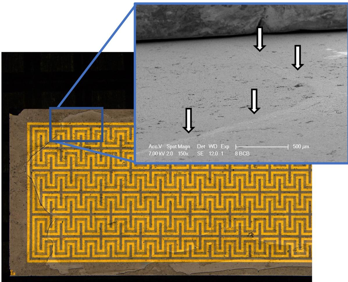
Figure 6.11: BCB zoom comparison with the fracture.
