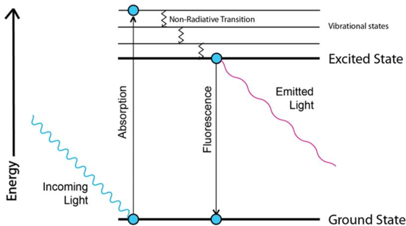
**Figure 5.2:** Working principle of fluorescence [19].
