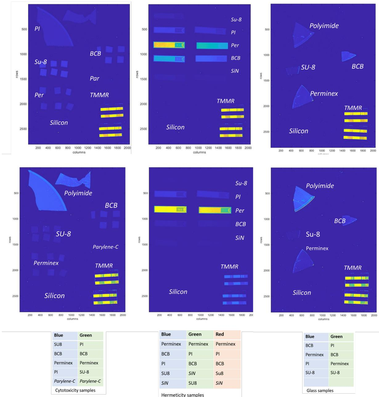
**Figure 5.21:** Overview of the images, with table of highest to lowest fluorescence of all equal polymer samples on one plate.
