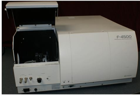
**Figure 5.4:** Image of the Hitachi FL-4500, the device the authors used to measure the fluorescence of BCB [23].
