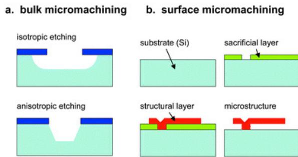
**Figure 2.1:** The difference between a.) Bulk micromachining and b.) Surface micromachining to produce the structure of a MEMS device.
