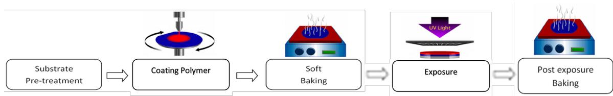
(b) Spin coating a polymer evenly on a wafer.
