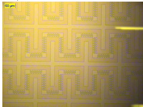
(c) The gold meander beams of the sample after lithography step (microscope).
