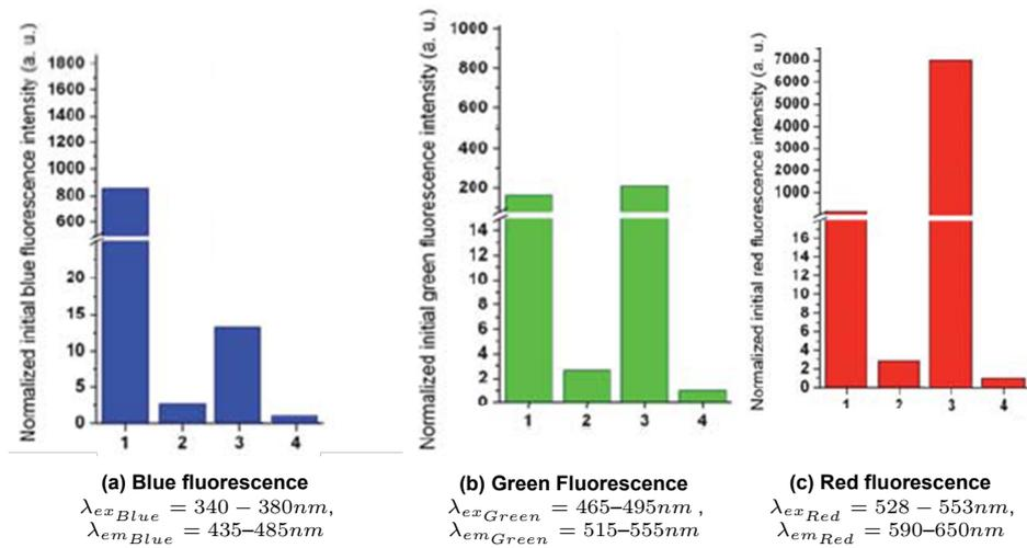
**Figure 5.6:** Fluorescence of (1): 5 mm parylene-C; (2): 380 mm PDMS; (3): 50.8 mm polyimide; (4): 980 mm Corning glass slide (control). This study made the corning glass slide the reference material, thus its auto-fluorescence of Corning glass microscope slide was set as 1 (a. u.). The values are normalized to 5 $\mu$ m thickness and all measurements were carried out with a 20x objective.
