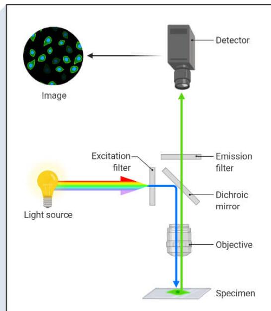
Figure 5.10: Schematic of the excited light passing through the microscope and if present how the fluorescent light passes to the detector of the microscope [29].
