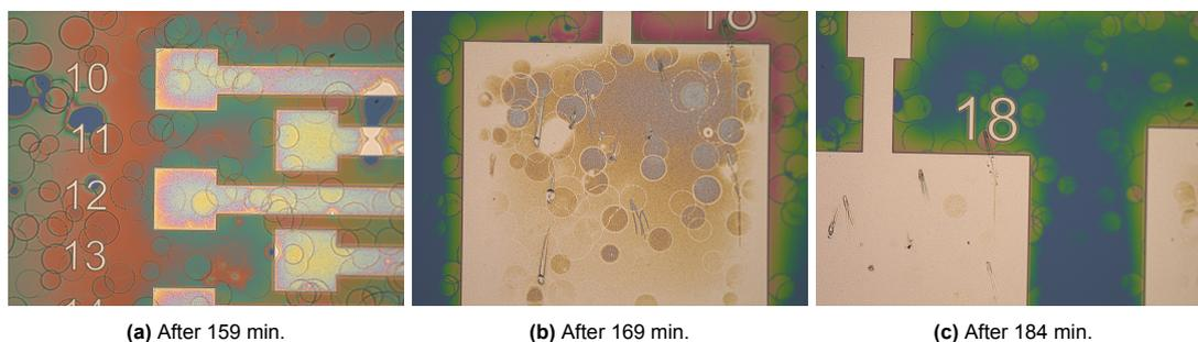
**Figure 7.3:** This figure shows the difference between steps in the barrel of a polyimide sample on aluminum tracks. It shows the result of an oxygen plasma (in time intervals of max 20min) after (Figure 7.3a) 159 min., (Figure 7.3b) 169 min. and (Figure 7.3c) 184 min.
