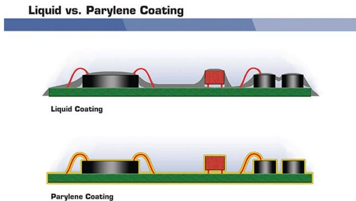
(a) Chemical vapour deposition, as the name suggests, the polymer will be deposited on the wafer when reactants are in vapour phase.
