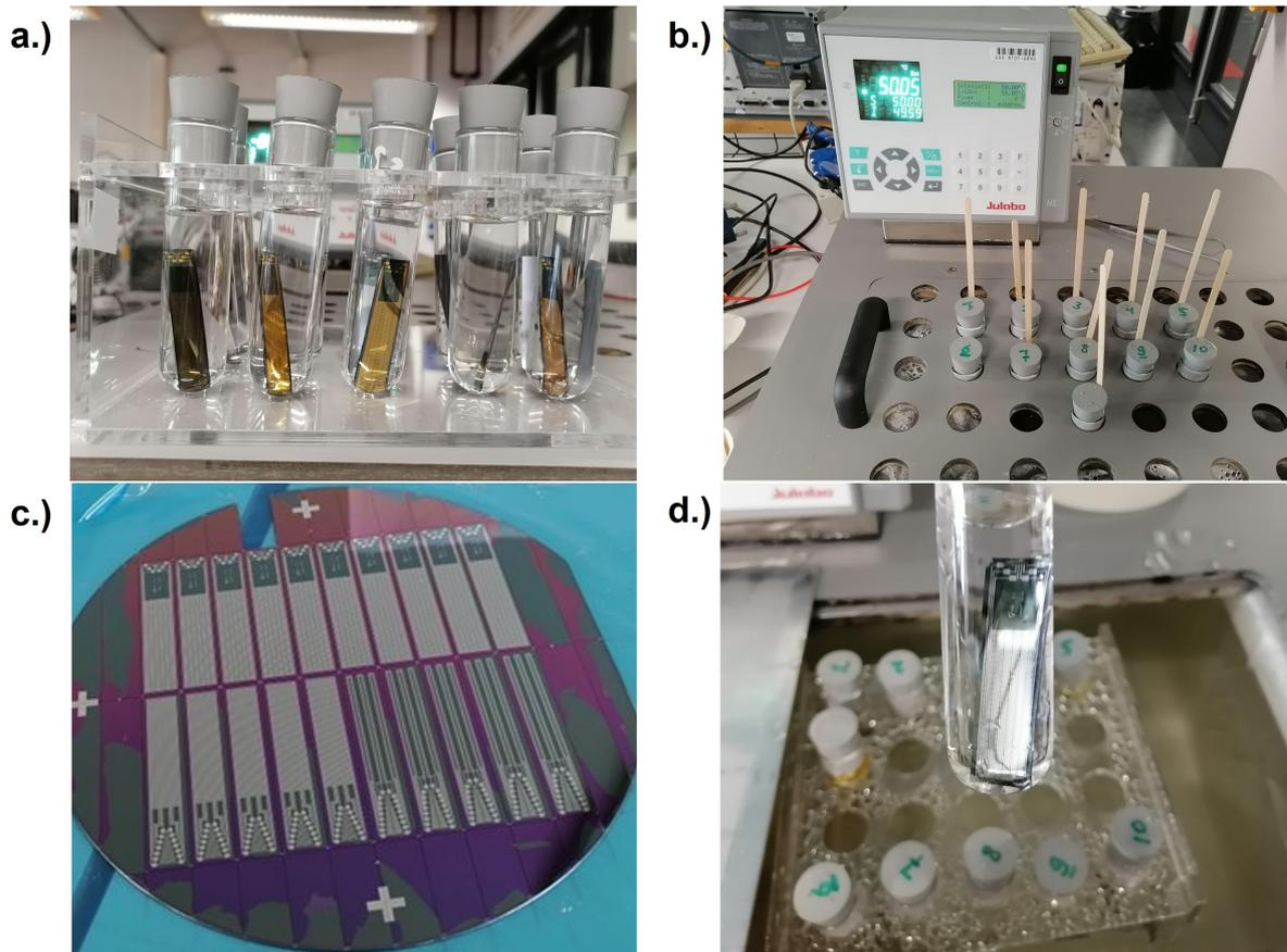
**Figure 6.2:** Hermeticity setup device and wafer: a.) Set-up of the pump in a box, with a cap. b.) SU-8 aluminum tracks wafer, after dicing. c.) Sample check on corrosion. d.) Aluminum samples in a tube with PBS.
