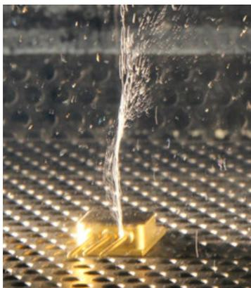
**Figure 6.1:** Image showing the leak of bubbles created by non-hermetic sealing
