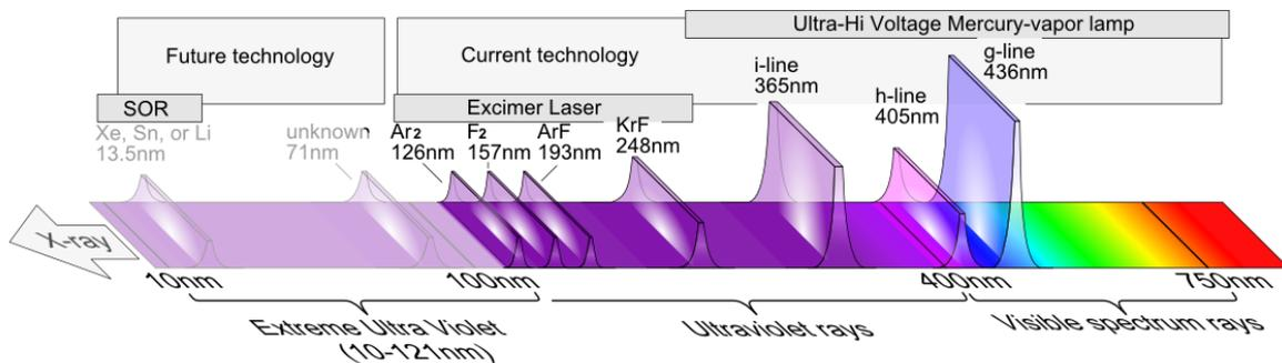
Figure 5.8: Spectrum for lithographic applications [26].
