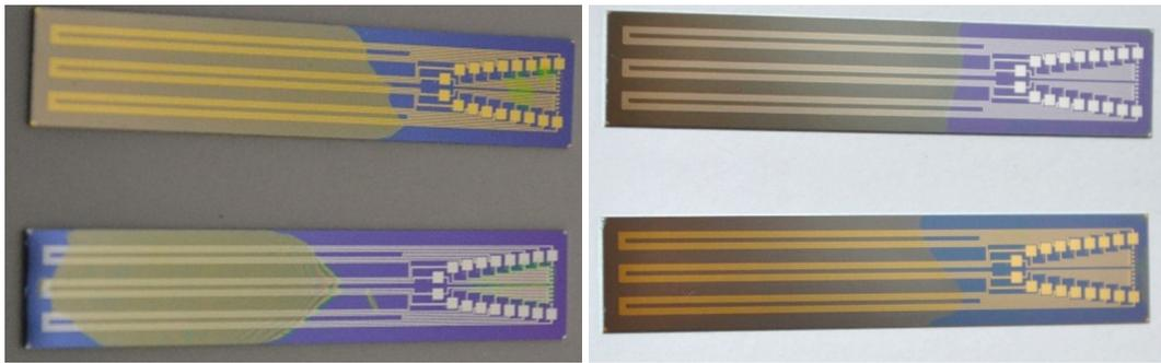
(a) Polyimide after oxygen barrel etch for a total of 179 minutes for gold and 184 minutes for aluminum. (b) Perminex samples after a 48 min. oxygen plasma and 20 min. extra.
