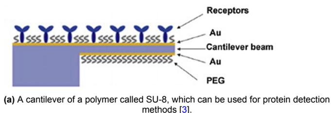
(a) A cantilever of a polymer called SU-8, which can be used for protein detection methods [3].
