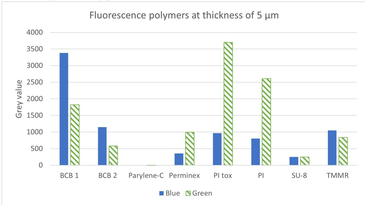
(b) Fluorescence of polymers (incl. TMMR) with correction for the background noise and normalized to 5 micrometers
