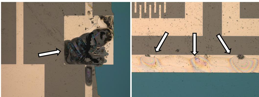
(a) Week 5: uncovered aluminum corroded.
