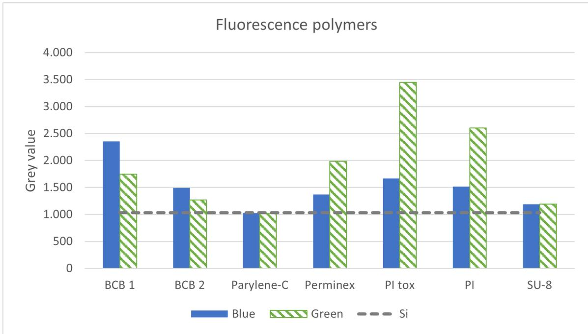
(a) Fluorescence of polymers with different thicknesses. TMMR excluded, value around 14.000 and 11.000.
