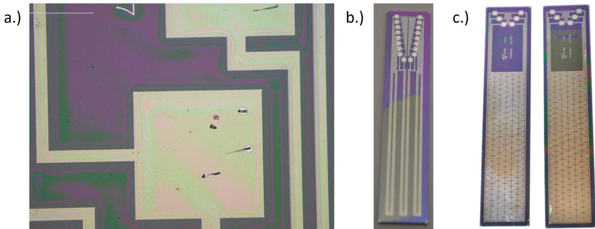
**Figure 7.5:** SU-8 results of layer removal tests. a.) SU-8 after an oxygen plasma etch time of 36 min. b.) SU-8 results after an oxygen plasma etch time of 48 min. c.) SU-8 results of cover test.
