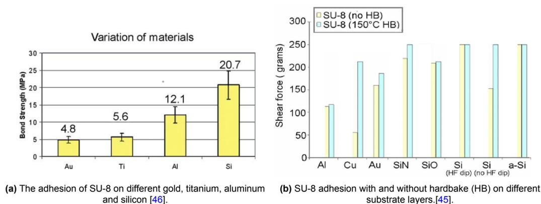
Figure 7.1: Adhesion of SU-8 on variety of substrate layers
