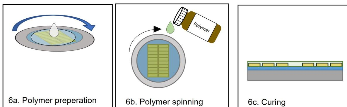
Figure 4.9: Polymer preparation, coating and curing.
