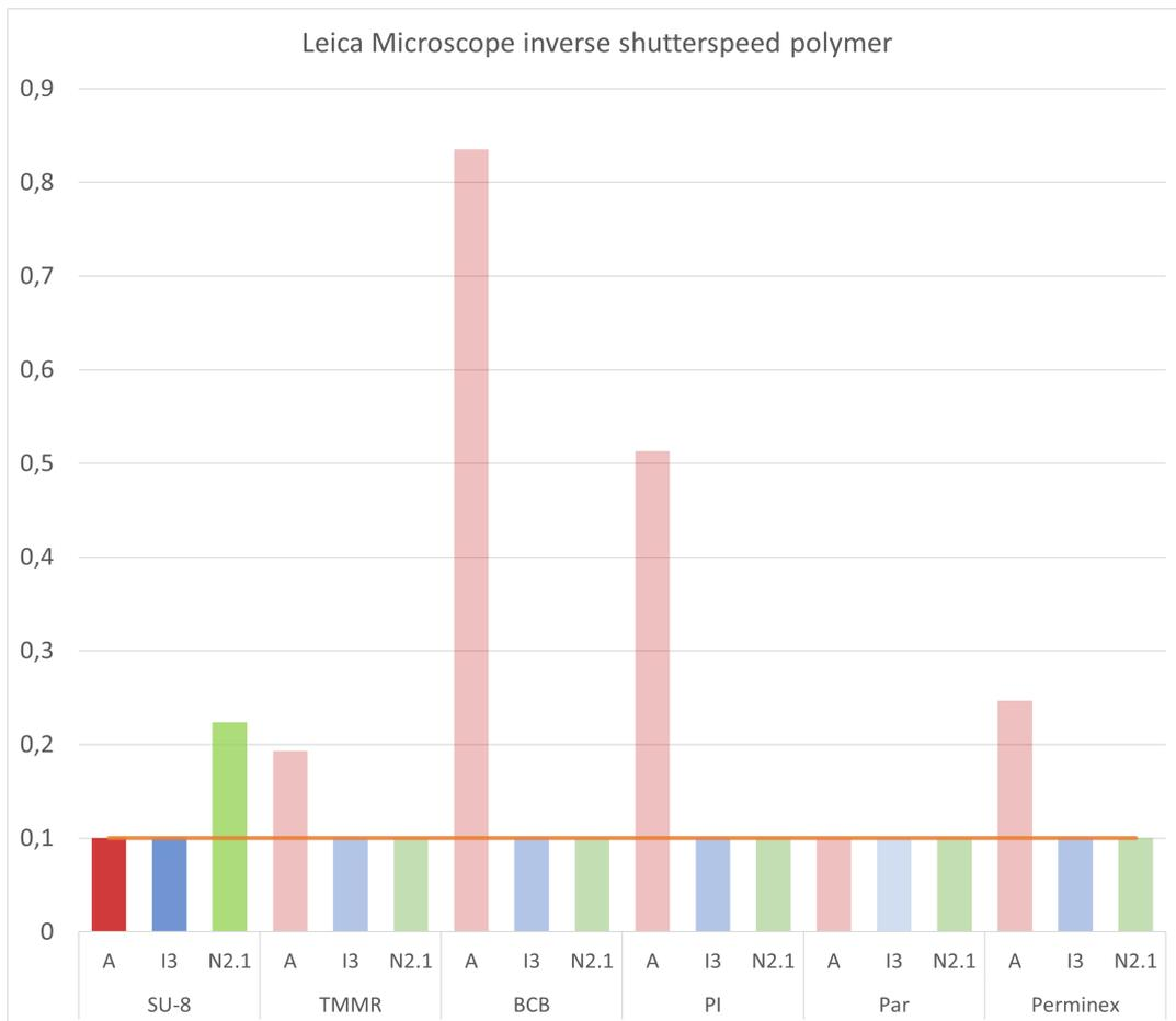
**Figure 5.17:** Inverse of the shutter speed measured with the Leica microscope on the polymer samples. (not normalized)
