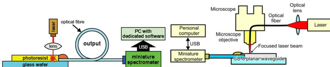
**Figure 5.3:** Scheme setup to measure the auto-fluorescence intensity with a laser. Left the setup of Microchem [21] and right the setup of P.Sniadek et al.[22].
