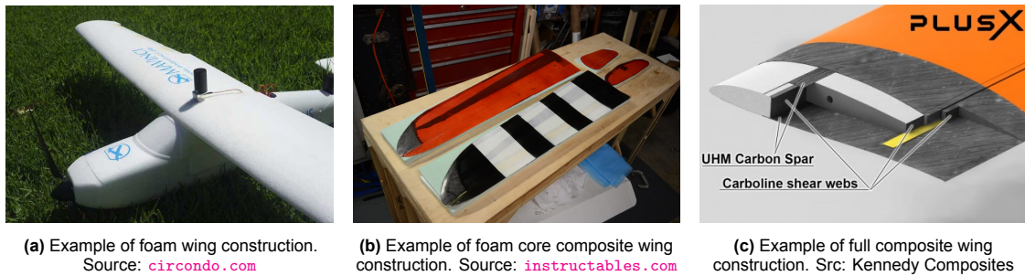
Figure 7.1: Various wing construction methods for small scale aircraft.
