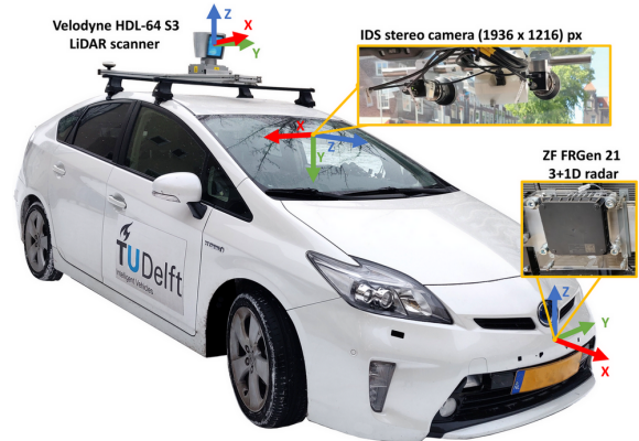
Fig. 2: Recording platform. Our Toyota Prius 2013 platform is equipped with a stereo camera setup, a rotating 3D LiDAR sensor, a ZF FRGen 21 3+1D radar, and a combined GPS/IMU inertial navigation system.
