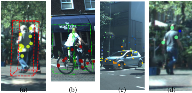
Fig. 7: Examples of incorrect detections by PP-radar : (a) merged smaller objects (two pedestrians are detected as a single cyclist), (b) larger objects split into smaller ones (one cyclist is detected as two pedestrians), (c) strong reflections and clutter nearby (metal poles and high curbs) and (d) distant objects with too few reflections (far away pedestrian).
