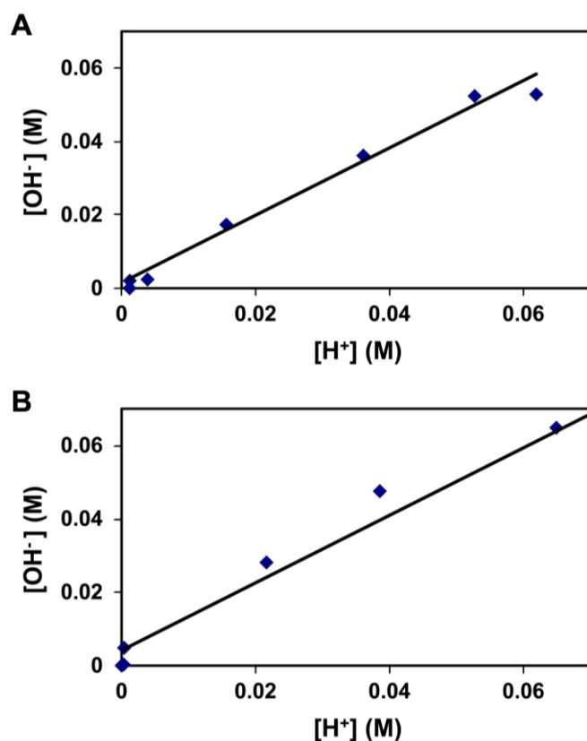
**Figure 4.6** Cumulative equivalent  $\text{OH}^-$  concentration (M) obtained from Ca ion released because of wollastonite dissolution vs. equivalent  $\text{H}^+$  released (M) by dissociated organic acids, in the biotic fed batch experiment (A). Cumulative equivalent  $\text{OH}^-$  concentration (M) obtained from Ca ion released because of wollastonite dissolution vs. equivalent  $\text{H}^+$  released (M) by HCl in the control 2 experiment (B).
