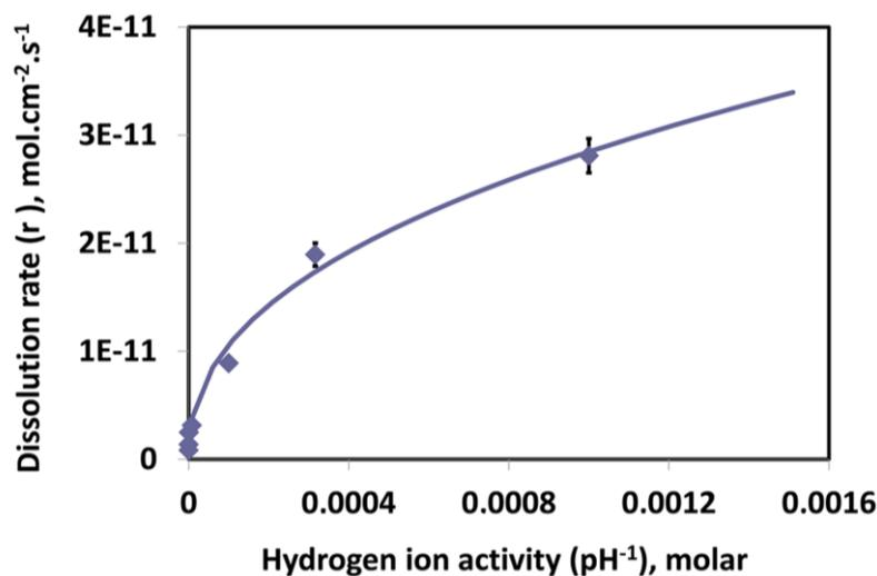
**Figure 4.3** Dissolution of wollastonite ( $\text{mol}\cdot\text{cm}^{-2}\cdot\text{s}^{-1}$ ) in chemical batch experiments at pH range of 3-8. The solid line represents the best fit of the data to the equation.
