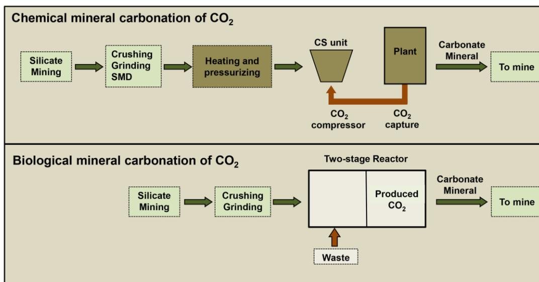
**Figure 2.5** Process comparison between biological and chemical mineral carbonation of CO<sub>2</sub>. The figure shows flow diagrams of a mineral carbonation of CO<sub>2</sub> by chemical methods and the proposed biological process. The processes of SMD for mineral pre-treatment, heating and pressurizing of the reactor, CO<sub>2</sub> capture, compression and transportation can be avoided as the result of integration into a biological treatment technology.
