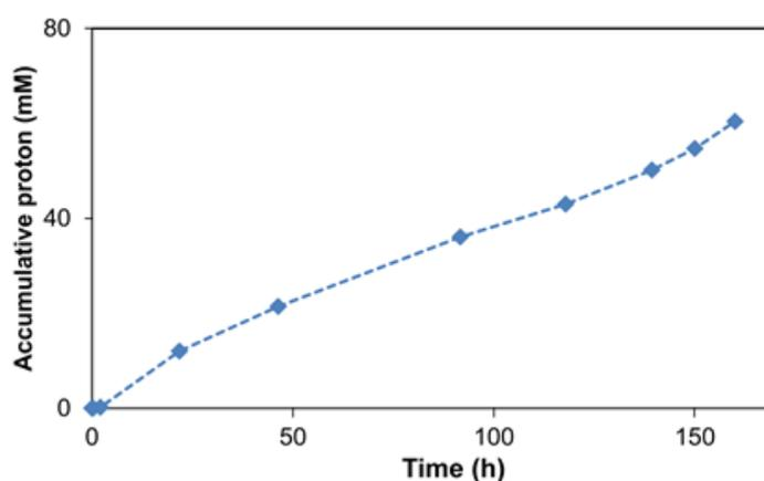
**Figure 4.7** The proton dosage rate in the abiotic fed-batch experiment (control 2) which was the same as in the control 1 experiment.
