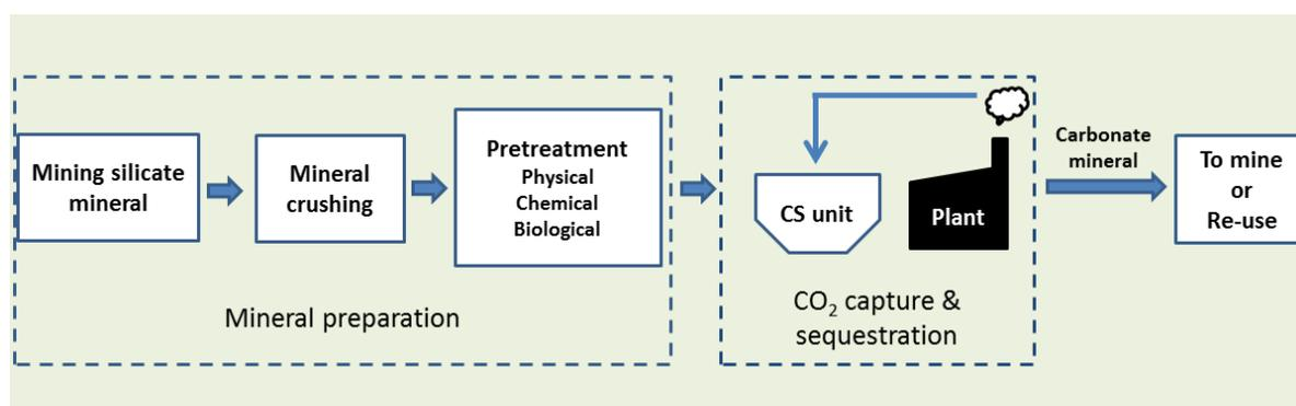
**Figure 1.2** Schematic drawing of a mineral CO<sub>2</sub> sequestration process. CS stands for carbon sequestration.
