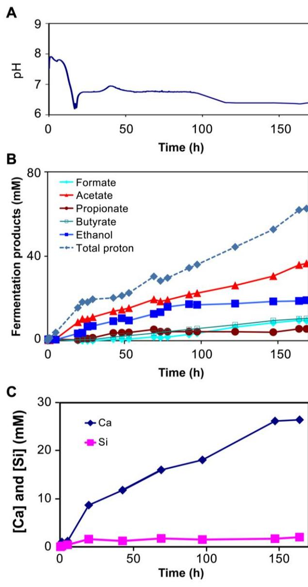
**Figure 4.4** Quantification of wollastonite dissolution kinetics in the biotic fed-batch reactor. The pH profile (A), the concentration of fermentation products (mM) and the total proton production (mM) (B), and cumulative concentrations of Ca ion and Si ion released by dissolution of wollastonite (C).
