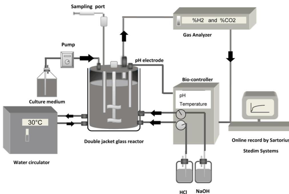
**Figure 4.2** Schematic setup of the biotic fed-batch reactor.
