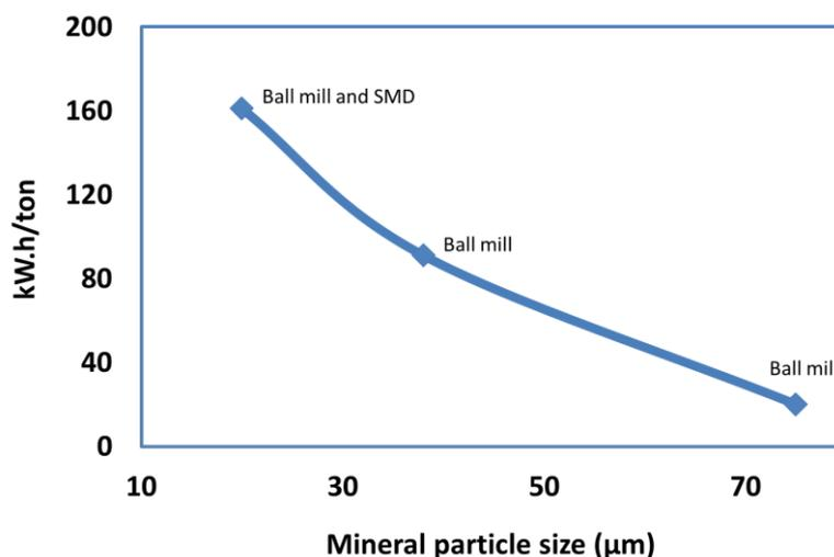
**Figure 1.3** The grinding energy required for size reduction of wollastonite particles. Adapted from (Gerdemann et al., 2007). This energy does not include the energy spent for mineral crushing. SMD stands for stirred media detritor.
