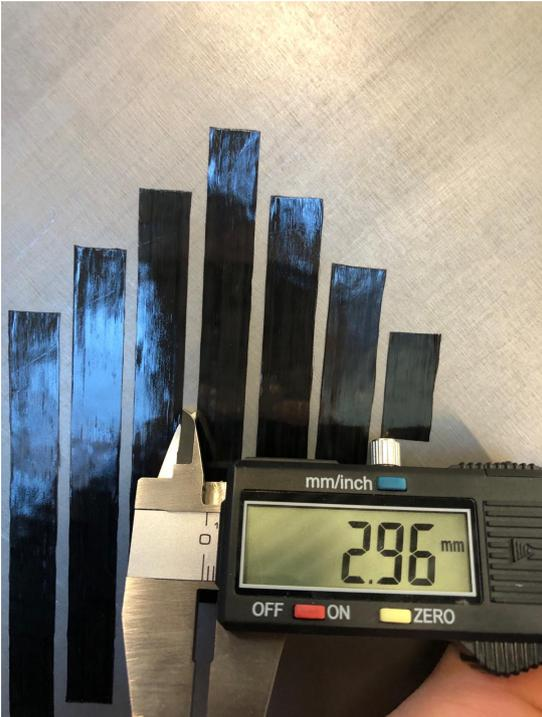
**Figure 5.4:** In-situ gap size measurement after lamination.
