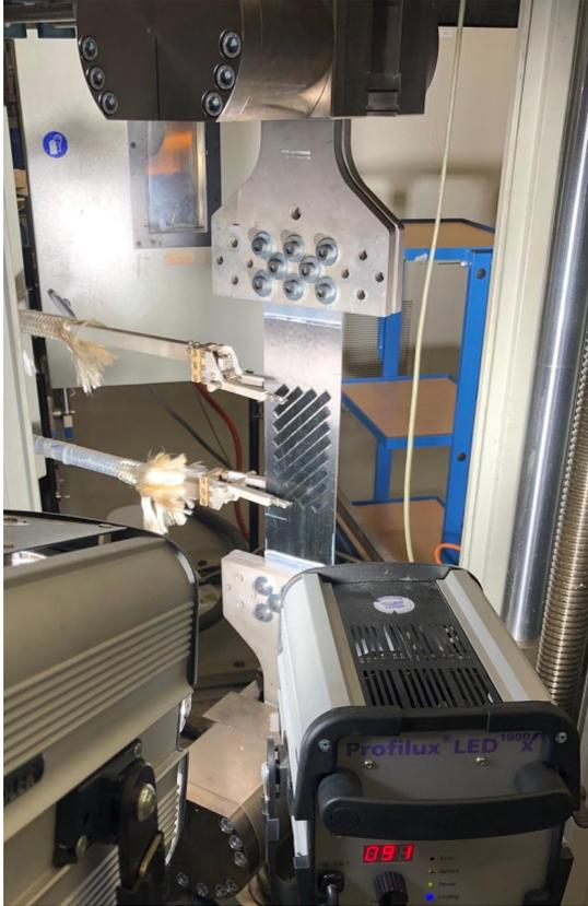
**Figure 5.17:** Clean specimen with clamping plates.
