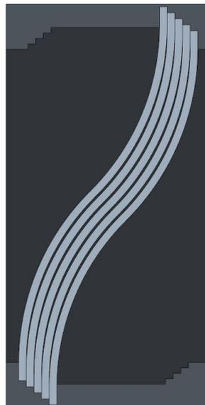
**Figure 4.8:** Second iteration of the initial concept without enveloping tows and extra clamping reinforcement.
