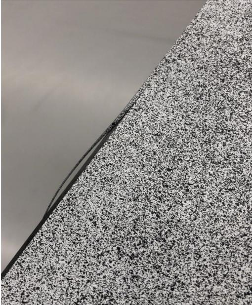
Figure 5.21: Delaminated strand at the edges of the specimen.
