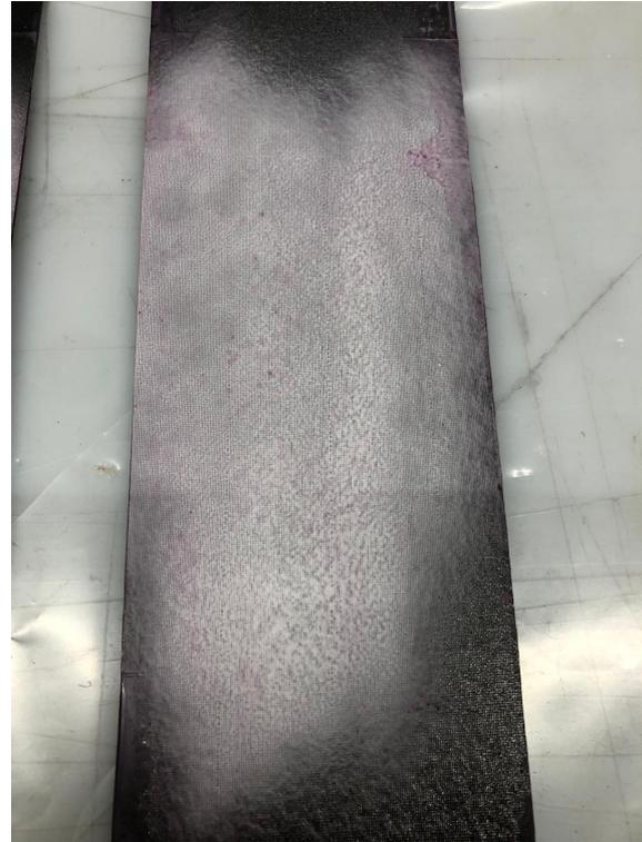
Figure 5.24: Rough side dye penetrant testing.
