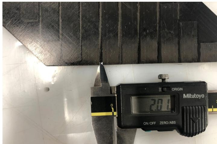
**Figure 5.11:** Cured gap size width of around 2 mm instead of the 3 mm set during lamination
