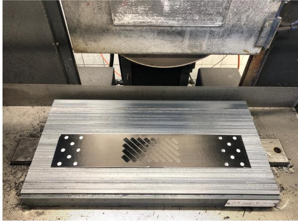
**Figure 5.13:** Cutting machine with a diamond blade used for the fine trimming of the specimen.
