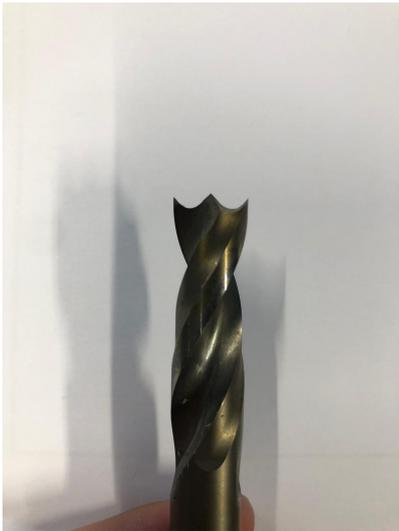
**Figure 5.12:** 'Brad point' drill bit used for the drilling of bolt holes.
