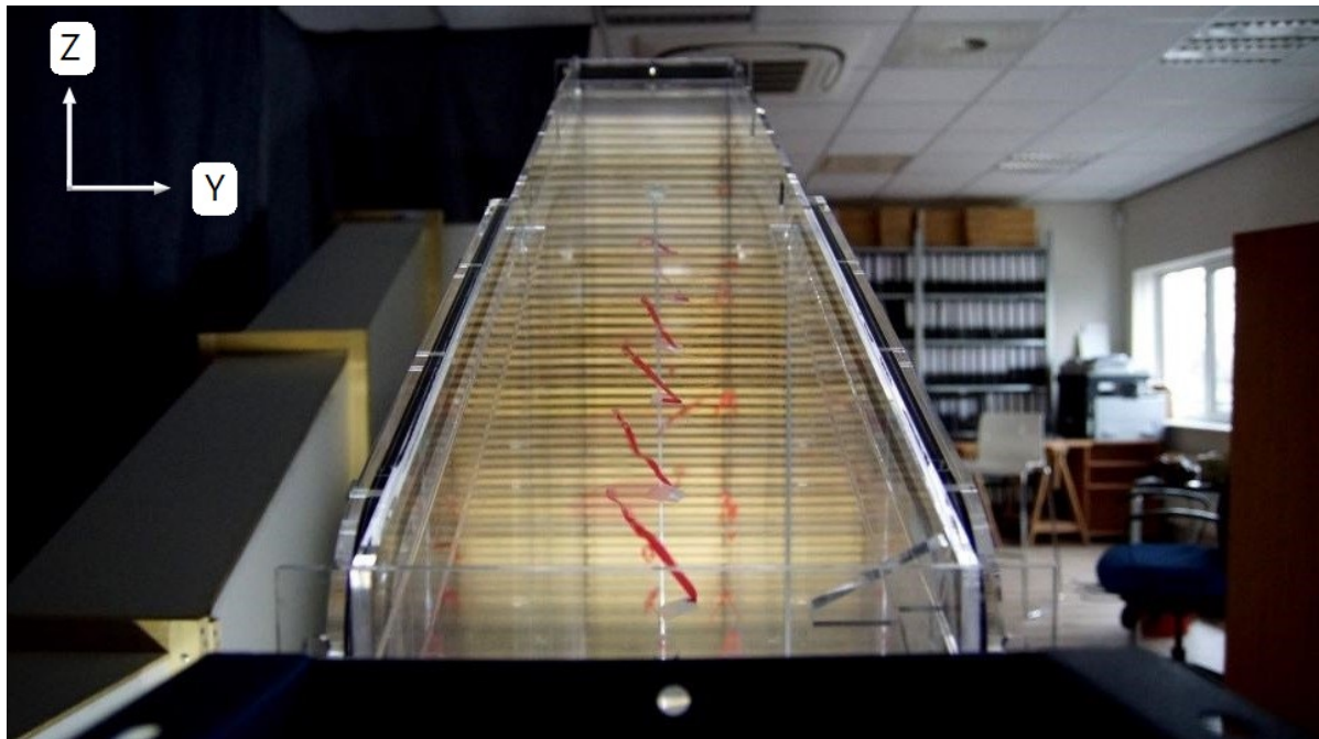
Figure 5.3: A view from the top surface of the diffuser. Note how the strips show that the jet, attached to the top surface, is swirling. This image was mirrored along its vertical centerline (and does not agree to other drawings of the windtunnel).
