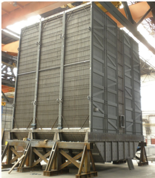
(a) Picture of a (flat) plate type heat exchanger, with application to air preheating of a fired heater.
