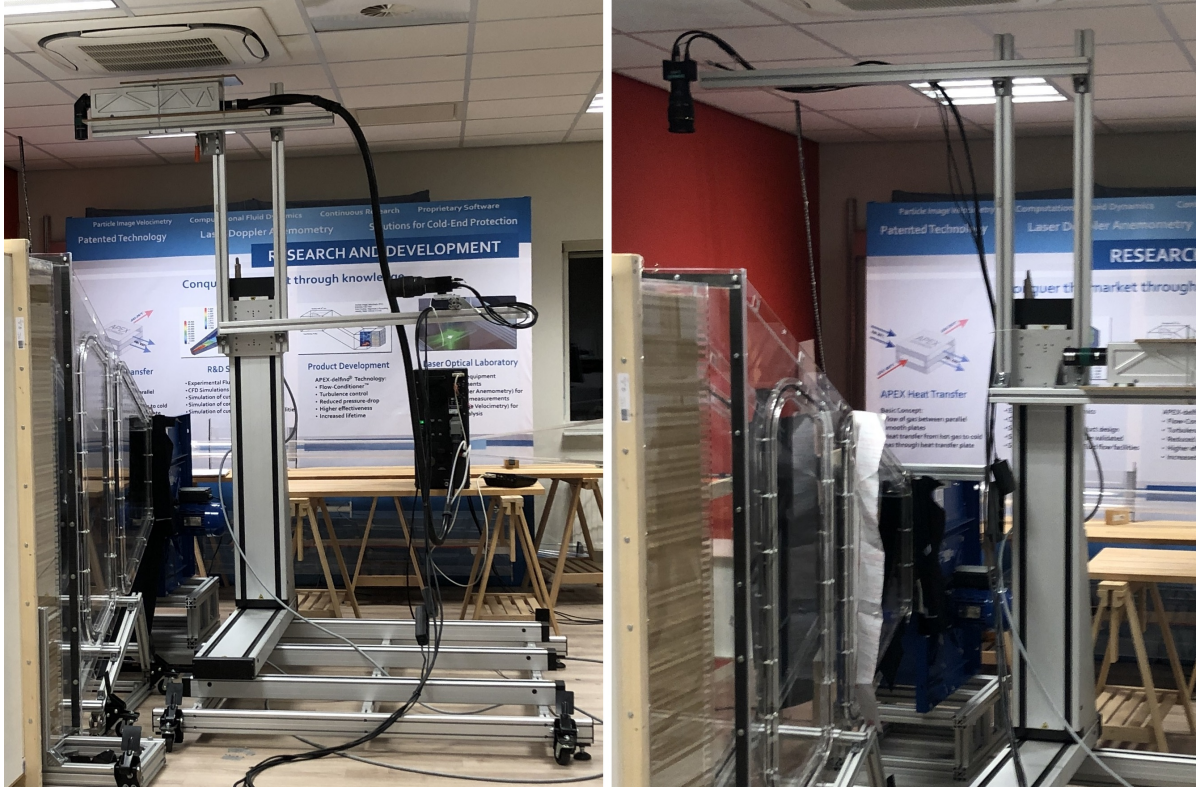
Figure 4.13: (left image) The requirement for a large focal length for the laser, resulted in the laser being mounted as high as possible. Before shutdown, the traverse would move to its fully up position, leaving only very small margins. (right image) Also when measuring in the horizontal planes, height was an important factor; the vertical distance between the camera and the light sheet had to be at least the height of the channel at the point where measurement were done.
