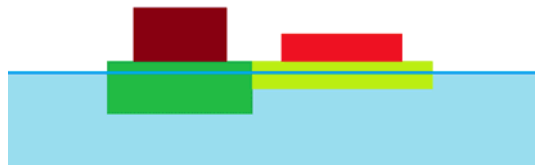
Figure 1: Floating structure with different superstructures and therefore different height floating body.
