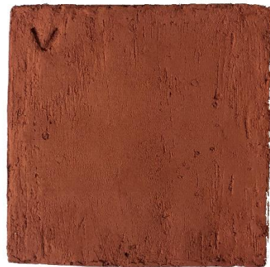
Figure 6: Example of a testing-tile that were made from crushed brick and clay to research its perfect composition, homogeneity, colour and texture.
