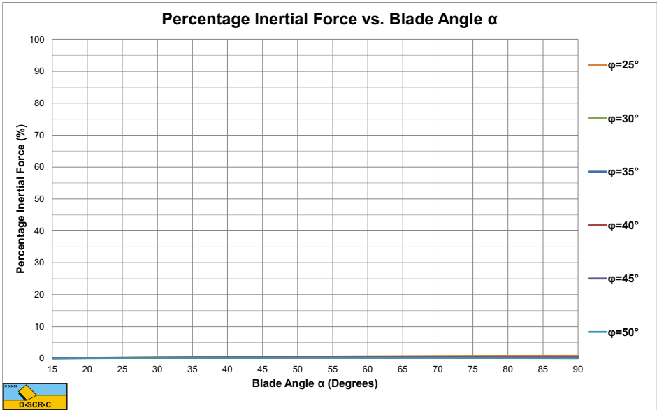
Figure B-19: The percentage inertial force for a dimensionless inertial effect parameter \lambda_i=0.025 .
