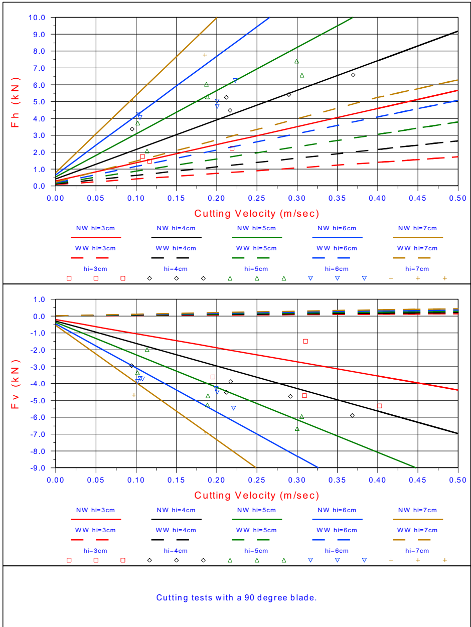
Figure 12-37: Cutting forces for cutting depths ( h_i ) from 3 to 7 cm; blade angle 90^\circ .
