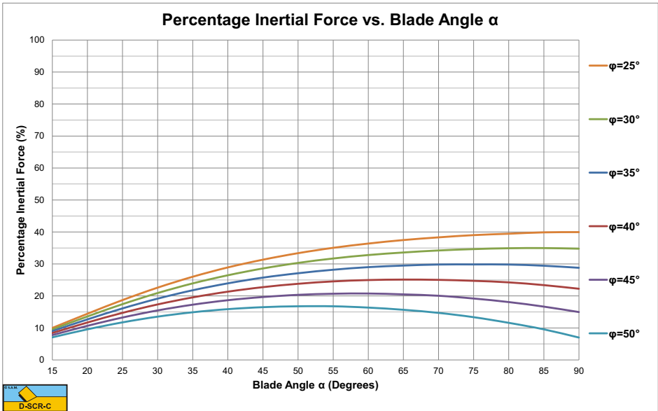
Figure B-21: The percentage inertial force for a dimensionless inertial effect parameter \lambda_i=2.5 .
