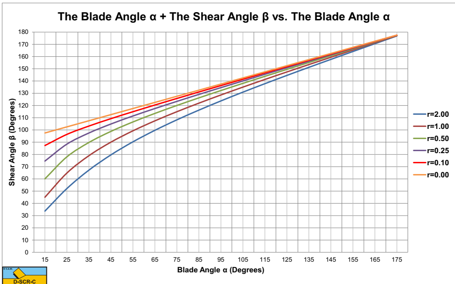
Figure 7-21: The blade angle \alpha + the shear angle \beta .
