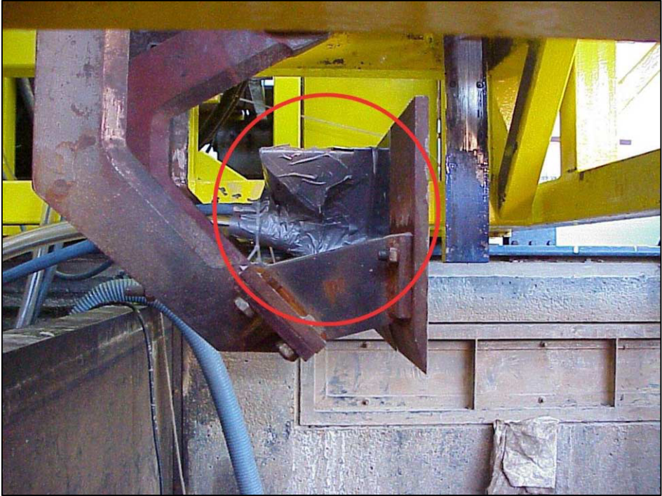
Figure 12-32: Cover with camera behind the blade.
