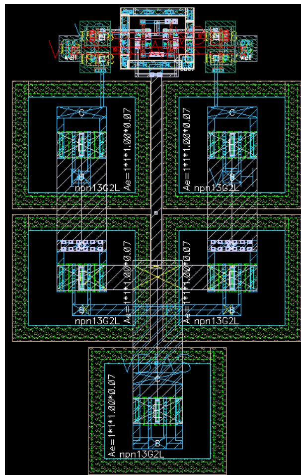
Figure 4.26: Layout view of the comparator
