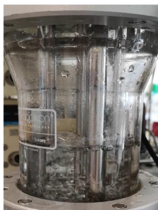
Figure S2. Photographs of bubbles in the STR with and without supplemented ethanol.
