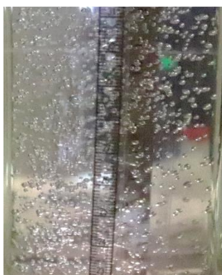
Figure S3. Photographs of bubbles in the BCR with mineral medium with and without supplemented ethanol. In the solution without ethanol, small but less stable, wobbling, bubbles were observed, while the ethanol leads to rigid, spherical, bubbles.
