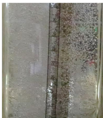
Figure S3. Photographs of bubbles in the BCR with mineral medium with and without supplemented ethanol. In the solution without ethanol, small but less stable, wobbling, bubbles were observed, while the ethanol leads to rigid, spherical, bubbles.
