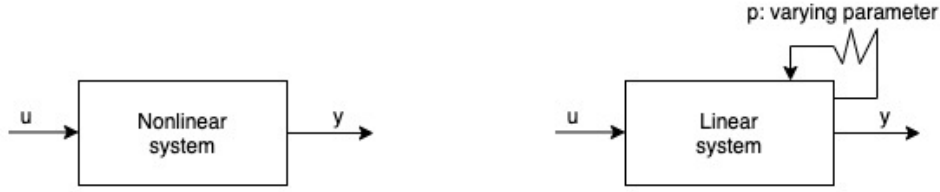
Figure 3.1: When using the LPV framework we can extract the scheduling variable p out of the system. When we extract this variable from the dynamics of the system we are left with a remaining relation between inputs and outputs that is linear.
