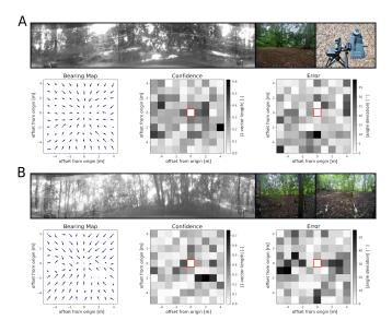
Fig. 7. Training performance in two real forest environments, one (A) open and bright and another (B) covered and dark. The images show grayscale training samples and an overview of the experimental area, along with experimental equipment and sample location markers (white arrows). Nest locations are shown in red.
