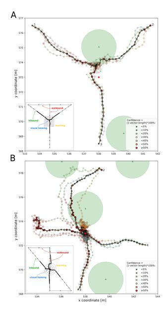
Fig. 6. Homing performance when controlling a simulated quadrotor based on a network trained on (A) a  $10 \times 10$  m grid and (B) an Archimedean spiral. Individual trajectories are shown transparent, with the mean trajectory per homing starting point in solid. Learning, outbound, inbound and visual homing phases are shown in the inset. Trees are shown in shaded green, and the nest is marked with a red cross at location  $\begin{bmatrix} 538, 573 \end{bmatrix}^T$ .
