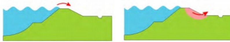
Figure 1.2: Failure mechanisms for the KIS project, left: overflow and overtopping right: macro stability inner slope Vergouwe et al. [2014]
