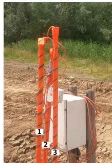
Figure 3.6: Intersection of piezometers in the subsoil (left) and measurement station at section W (right)
