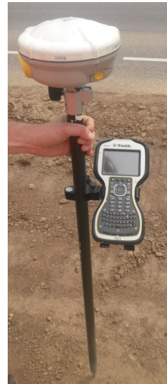
Figure 3.5: GPS surveying system: Trimble R8 GNSS System
