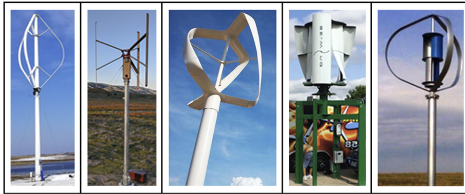
Figure 13. Common VAWT archetypes found on the current DWT market. From left to right: Darrieus Troposkien (photo credit: Chava Wind), H-Darrieus (photo credit: Xflow Energy), H-Darrieus with helix shape (photo credit: PRAMAC), Savonius (photo credit: BE Wind), combined Savonius–Darrieus (photo credit: HiVAWT).
