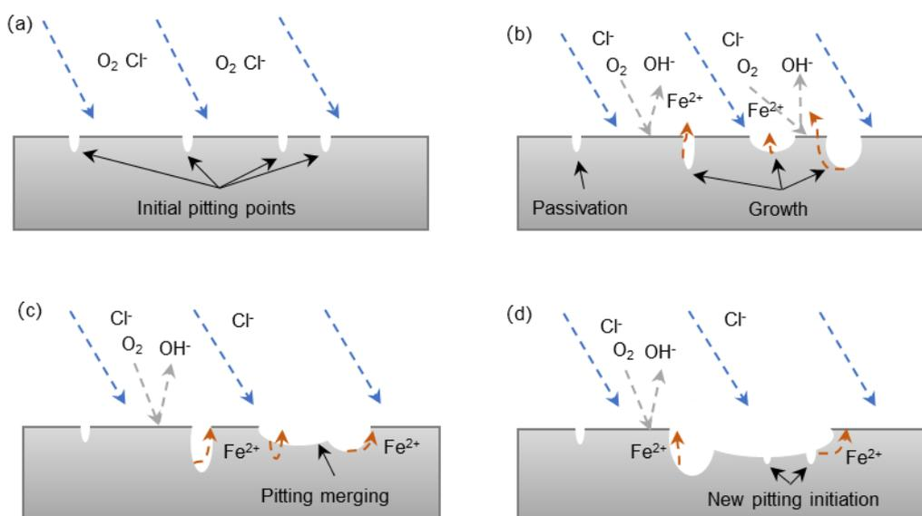
Figure 26 Schematic diagram of the corrosion process of the matrix of MC steel in NaCl solution from the cross-sectional view
