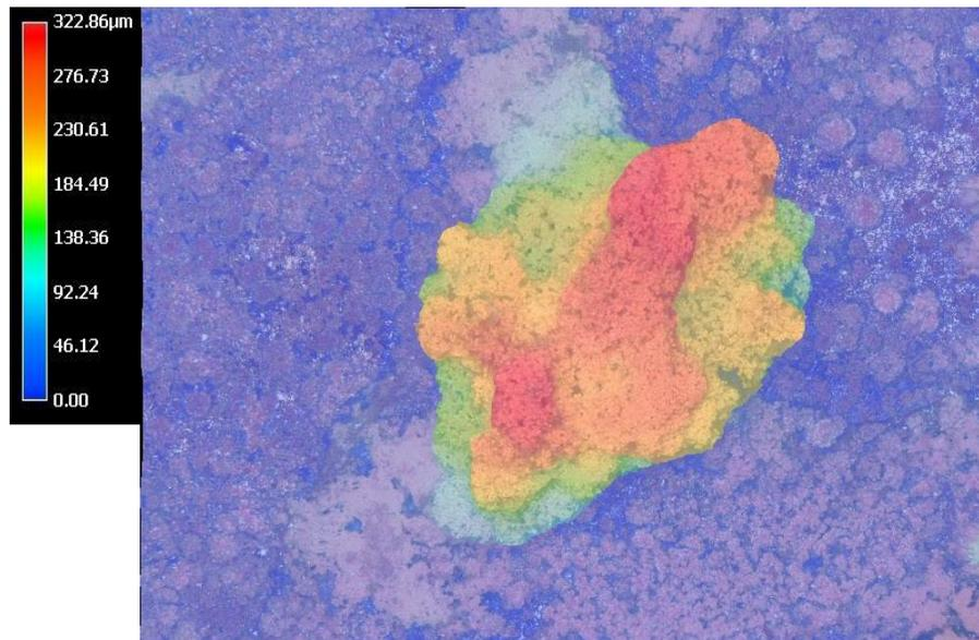
Figure A. 4 The height difference of microstructure of MC steel in NaCl solution without accelerating potential
