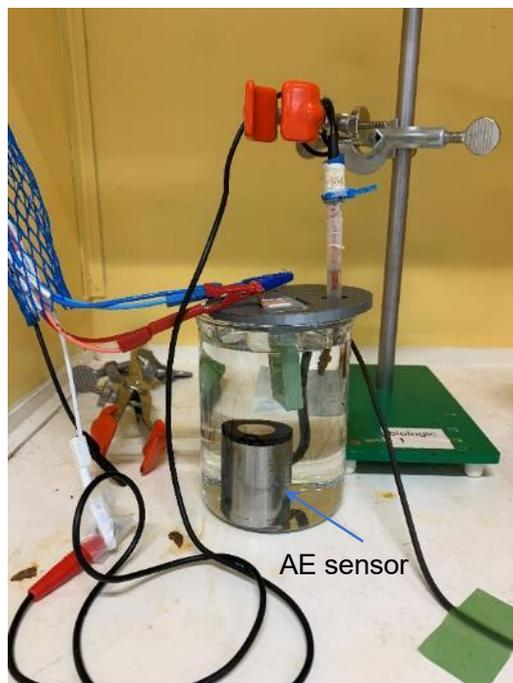
Figure A. 2 Setup in AE monitoring experiments
