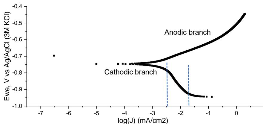
Figure 12 Potentiodynamic polarization curve obtained for the MC steel in 3.5 wt.% NaCl solution
