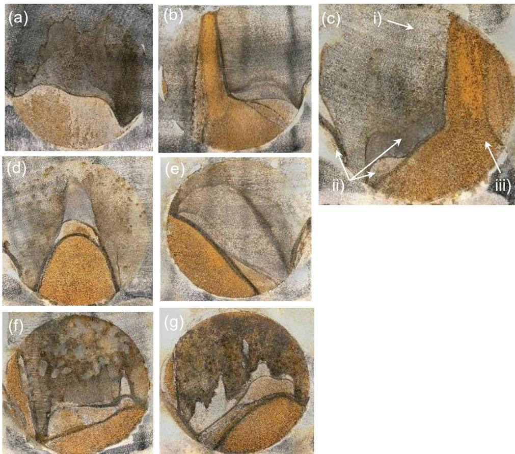
Figure 16 The evolution of the macro morphology of MC steel in NaCl solution with different immersion days: (a) 1 day; (b) 2 days; (c) 3 days; (d) 4 days; (e) 5 days; (f) 6 days; (g) 7days
