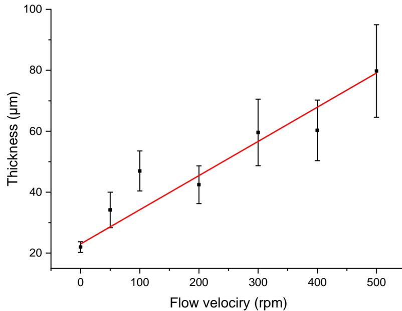
Figure 32 The thickness of the rust layer of MC steel in 3.5 wt.% NaCl solution at different flow velocities
