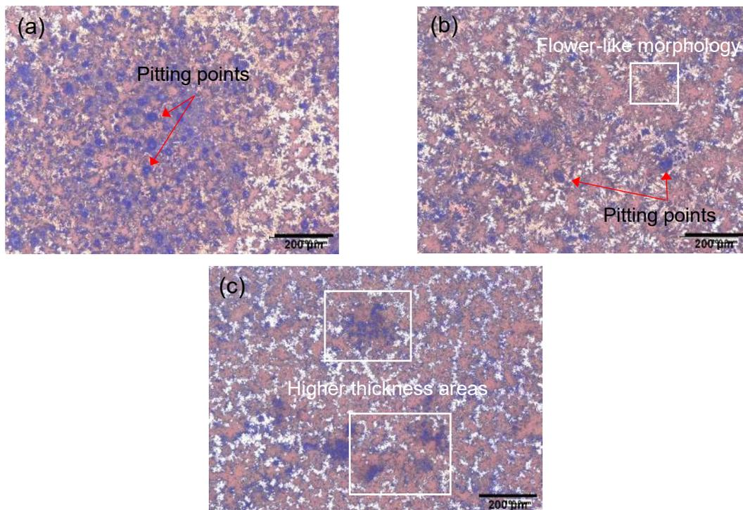
Figure 40 The morphology of rust layer of the sample at different temperatures: (a) 10 °C; (b) 15 °C; (c) 25 °C
