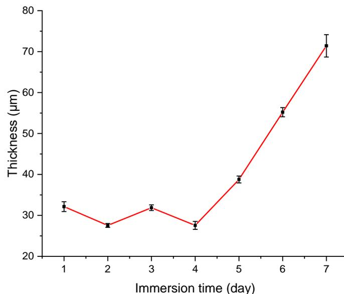
Figure 18 Time dependence of the thickness of rust layer for MC steel in 3.5 wt.% NaCl solution
