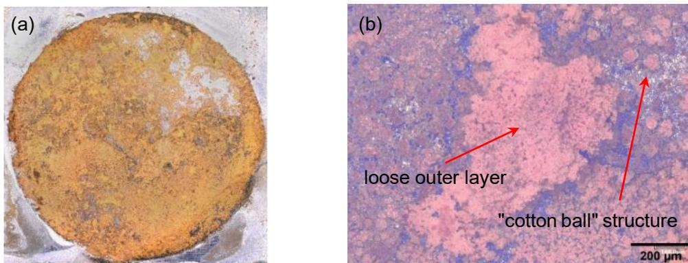
Figure 23 The morphology of MC steel in NaCl solution without accelerating potential (a) macrostructure; (b) microstructure at  $\times 300$  magnification
