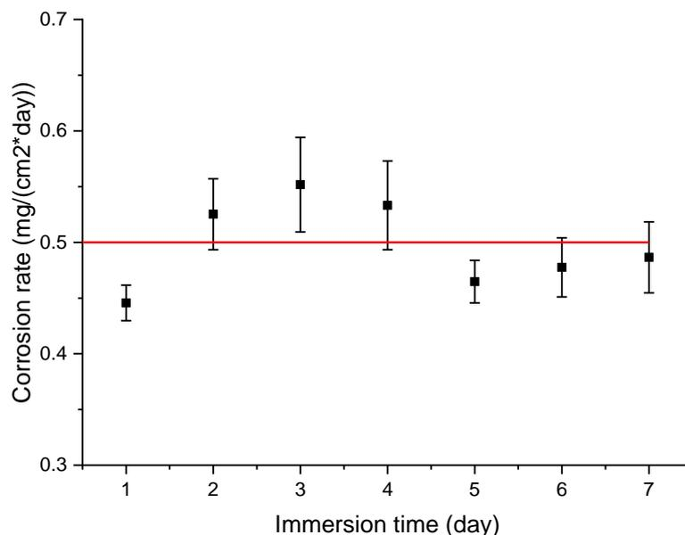
Figure 15 The corrosion rate of MC steel in 3.5 wt.% NaCl solution
