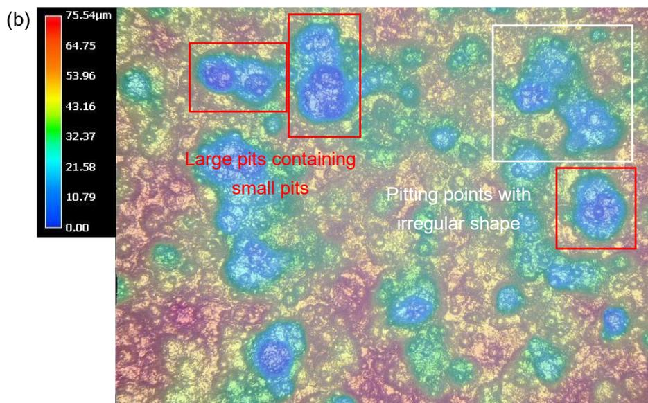
Figure A. 5 The height difference of microstructure of MC steel in NaCl solution (a) with accelerating potential (b) with OCP at  $\times 200$  magnification
