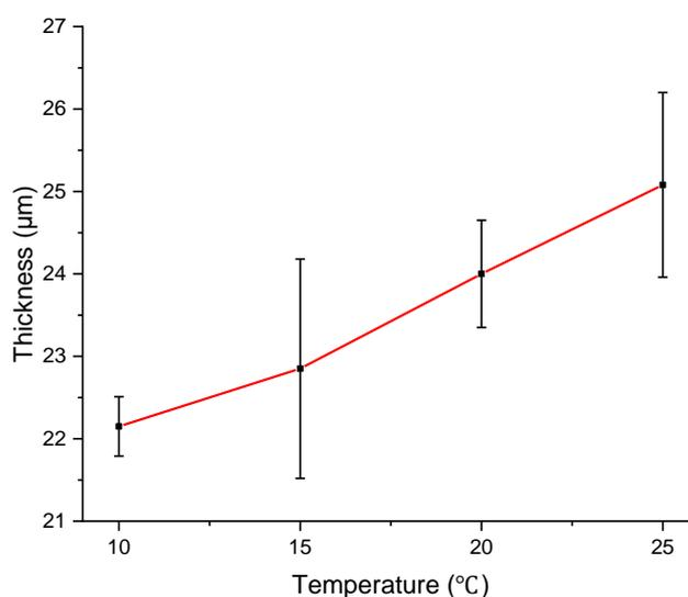
Figure 41 The thickness of the rust layer of MC steel in 3.5 wt.% NaCl solution at different temperature
