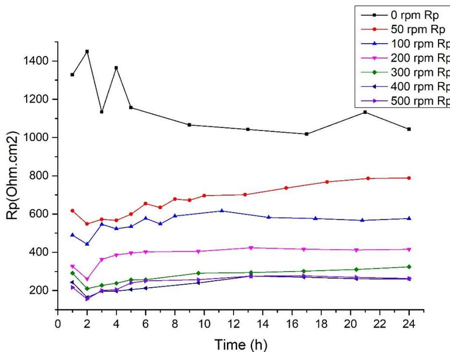
Figure 28 Time dependence of  $R_p$  for MC steel in 3.5 wt.% NaCl solution at different flow velocities
