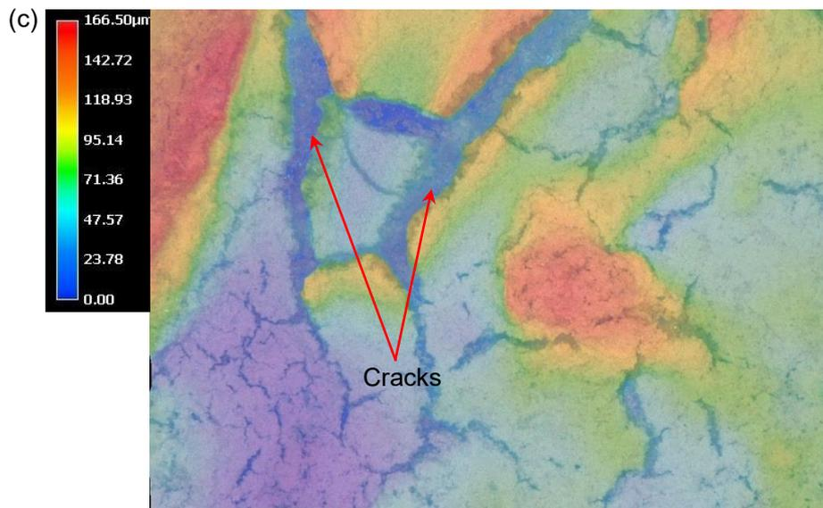
Figure A. 7 The height difference of the rust layer on the sample with (a) 50 rpm; (b) 100 rpm; (c) 500 rpm flow velocity
