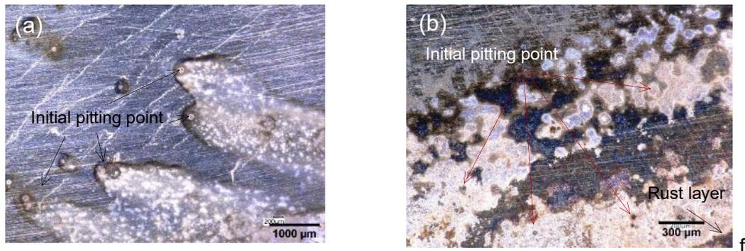
Figure 17 Observation by digital optical microscopy of a low-corrosion area of a sample immersed for 4 days in 3.5 wt.% solution under (a) $\times 50$ ; (b) $\times 150$  magnification
