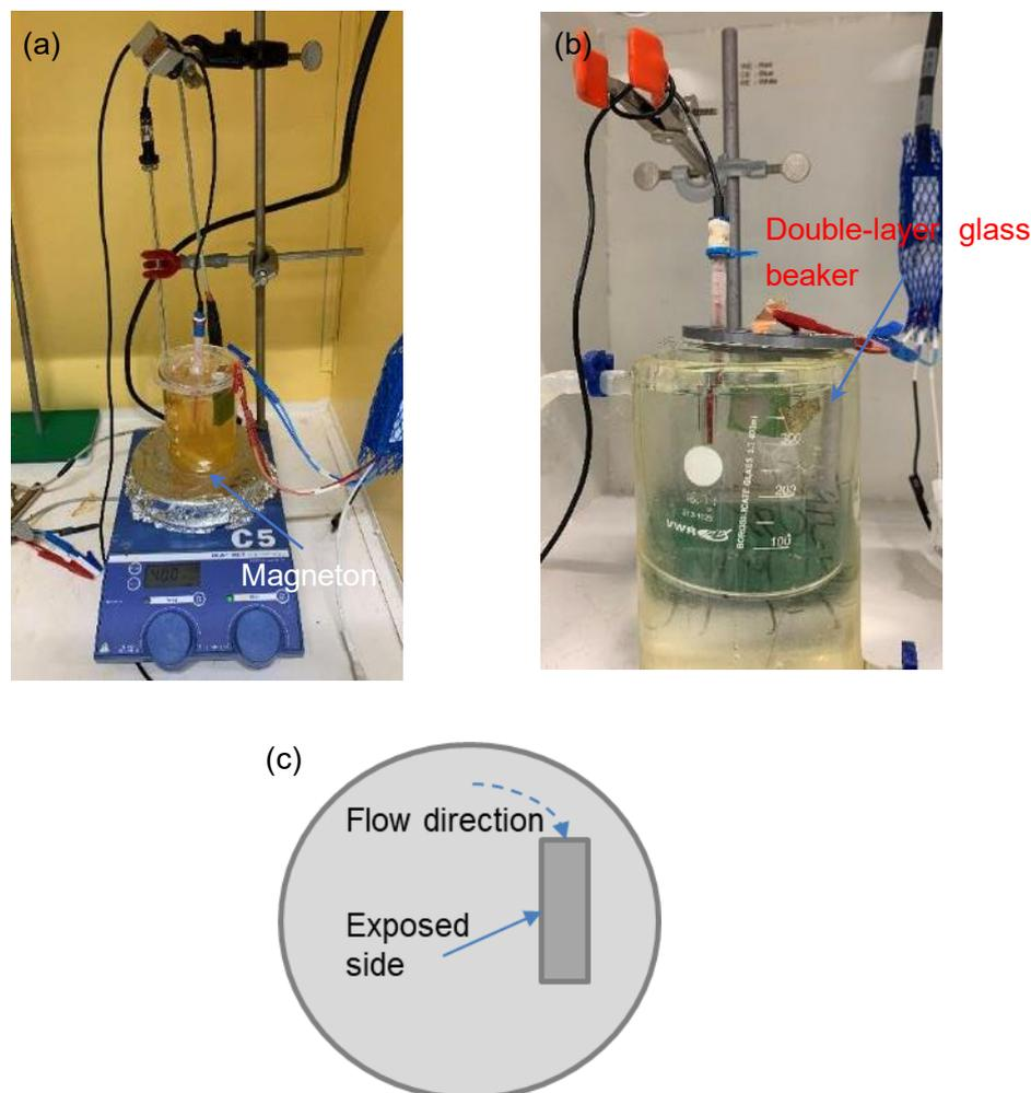
Figure A. 1 Electrochemical detection setup in the experiments to study the influence of (a) flow velocity; (b) temperature; (c) Schematic diagram of sample placement in flow velocity experiments
