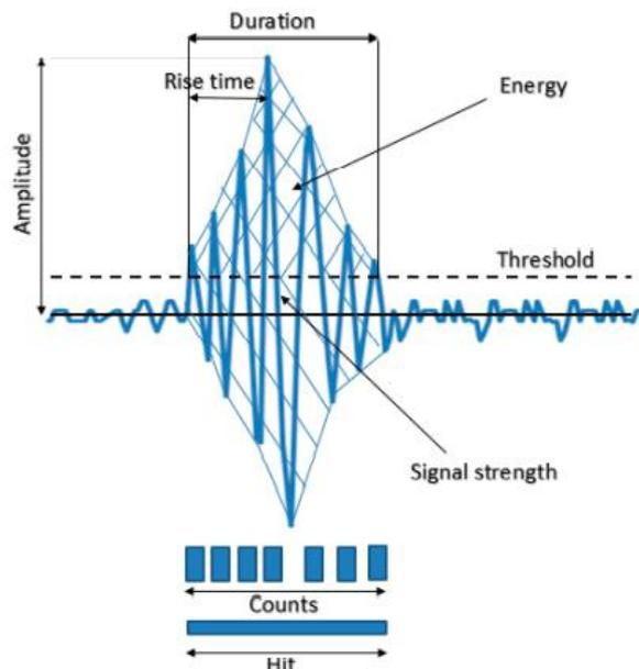
Figure 10 Parameters reflecting of an AE waveform
