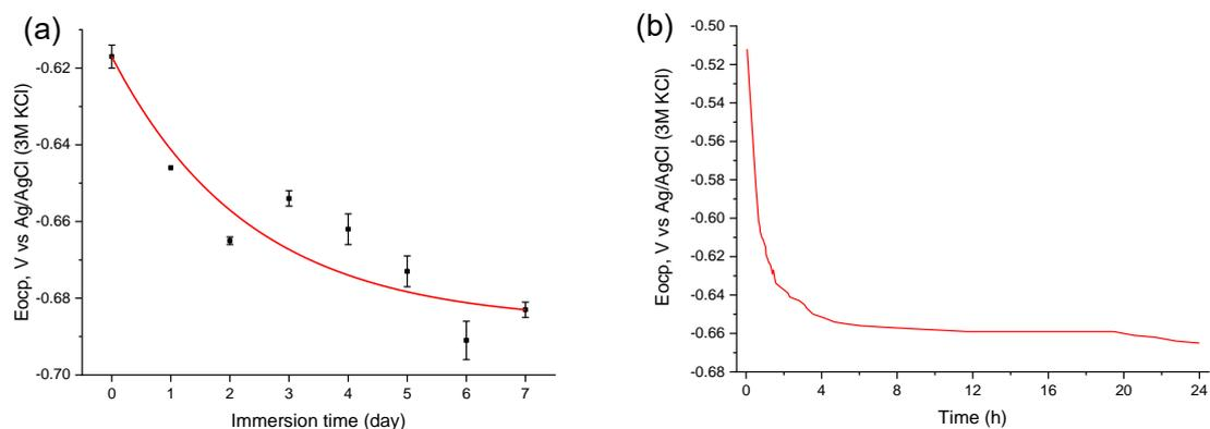
Figure 13 Evolution of  $E_{OCP}$  with the time of MC steel in 3.5 wt.% NaCl solution: (a) in the first day; (b) in one week
