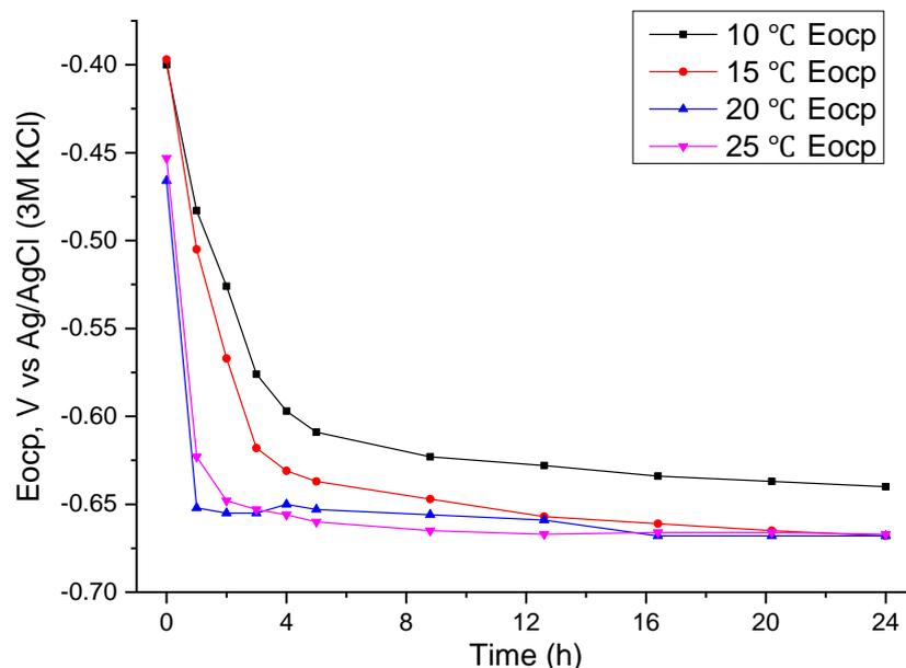
Figure 35 Evolutions of  $E_{OCP}$  of MC steel in 3.5 wt.% NaCl solution at different temperature
