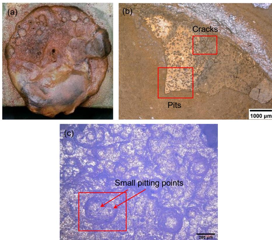
Figure 24 The morphology of MC steel in NaCl solution with accelerating potential (a) macrostructure of outer rust layer; (b) macrostructure of inner rust layer; (c) microstructure at  $\times 200$  magnification
