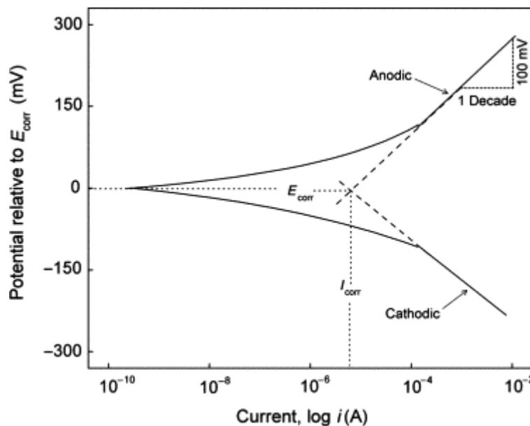
Figure 7 Schematic polarization curve with Tafel extrapolation [58]
