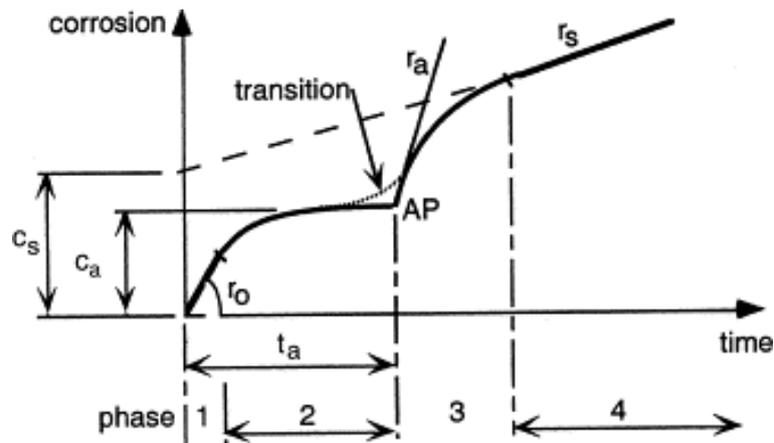
Figure 4 Mean-value corrosion loss as a function of exposure time for uniform corrosion freely rendered from [22]
