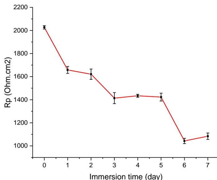
Figure 14 Time dependence of  $R_p$  for MC steel in 3.5 wt.% NaCl solution
