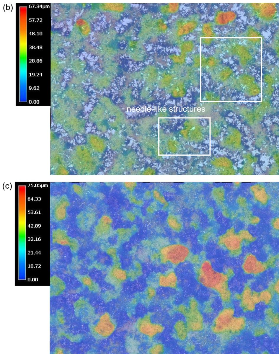
Figure A. 3 The height difference of morphology of rust layer immersed for (a) 1 day; (b) 4 days; (c) 7 days
