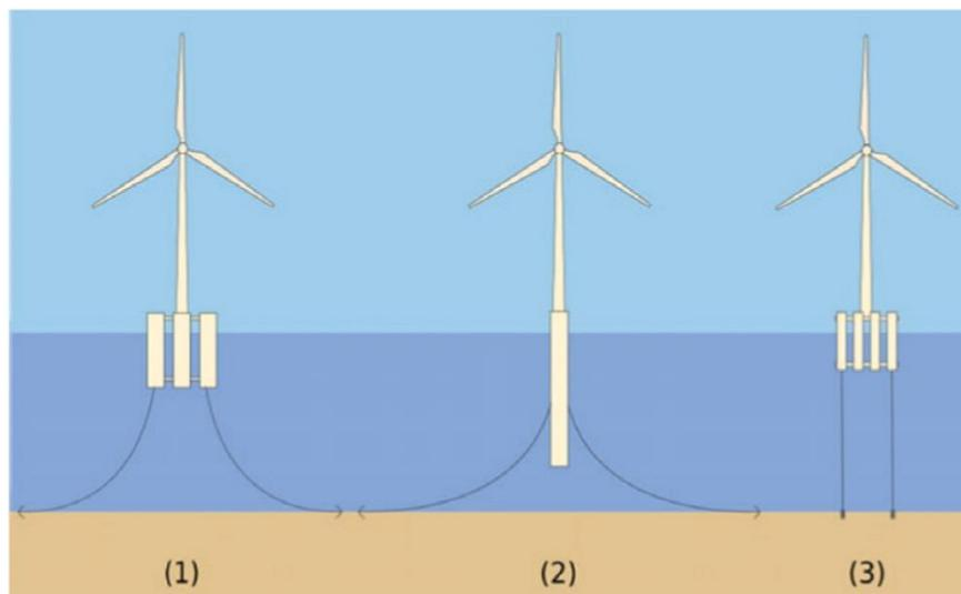
Figure 1 Floating wind turbine structures: (1) semi-submersible platform; (2) spar; and (3) tension leg platform (TLP) freely rendered from [1]
