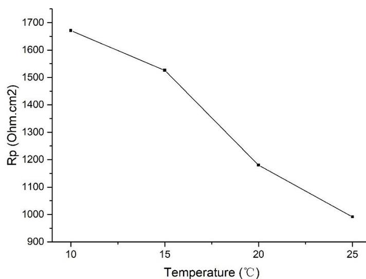
Figure 37 The evolution of final  $R_p$  at different temperature
