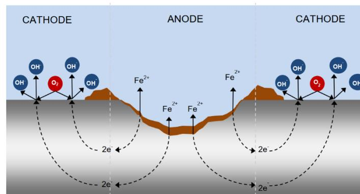
Figure 3 Schematic of the corrosion process and the presence of water is implied freely rendered from [20]
