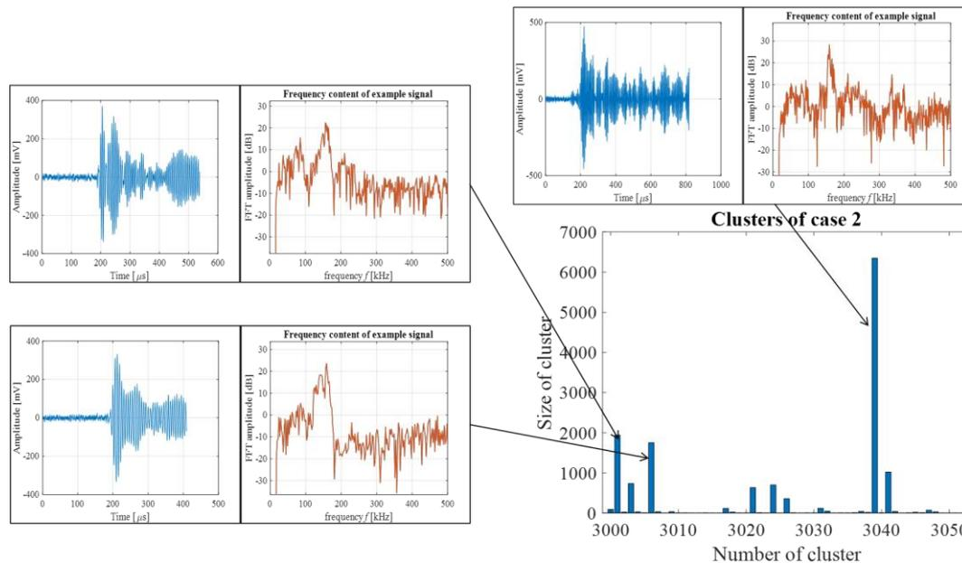
Figure 21 The clustering diagram of Case 2 and the representative signals of the three peaks with the largest number
