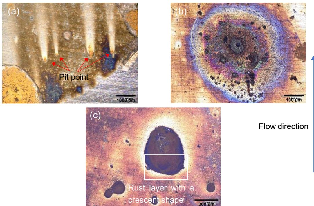
Figure 33 The morphology of low-corrosion area of the sample with (a), (b) 50 rpm; (d) 100 rpm flow velocity (water flows from bottom to top)
