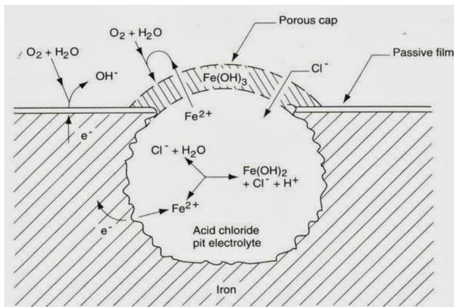
Figure 5 Autocatalytic process occurring in a pitting location freely rendered from [45]
