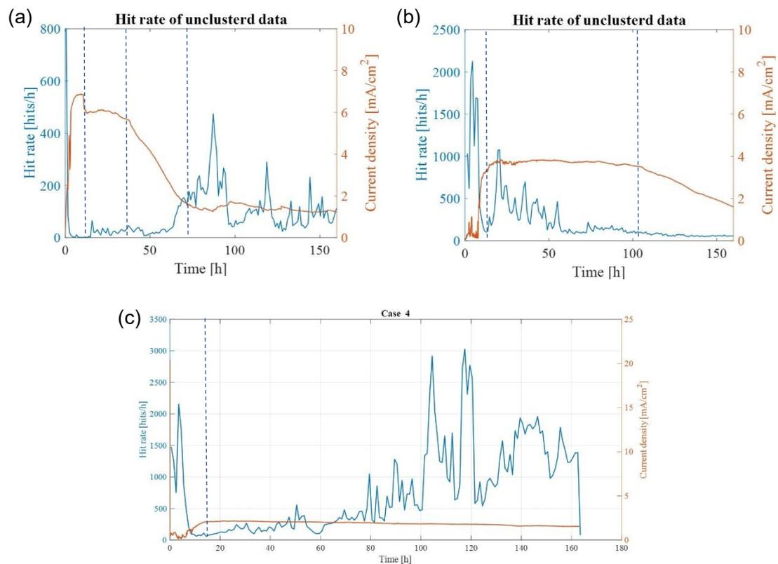
Figure 20 Schematic diagram of current density and hit rate of modified AE signals vs time for (a) Case 2; (b) Case 3; (c) Case 4
