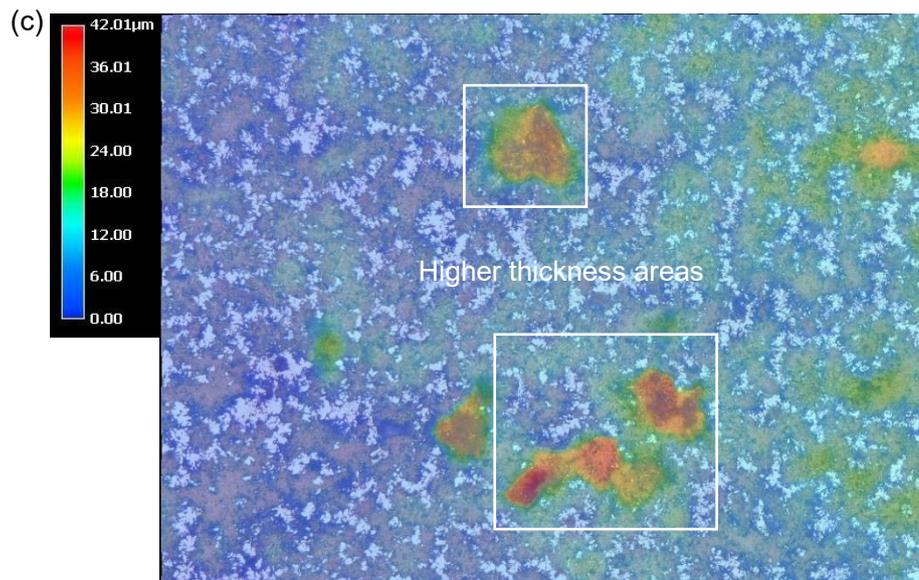
Figure A. 8 The height difference of the rust layer on the sample at different temperatures: (a) 10 °C; (b) 15 °C; (c) 25 °C
