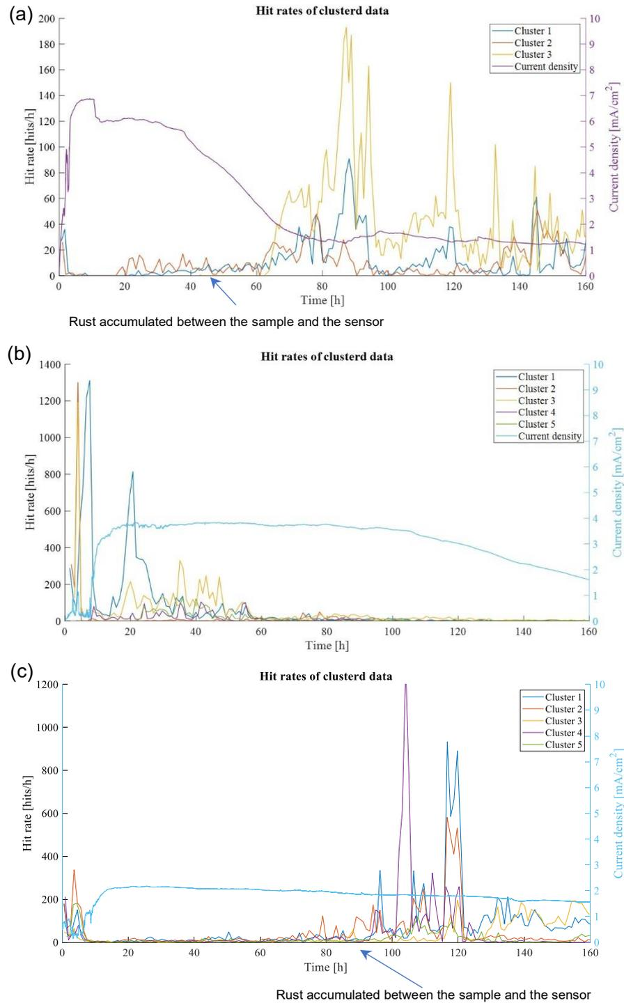
Figure 22 Schematic diagram of clustered hit rate of modified AE signals vs time for (a) Case 2; (b) Case 3; (c) Case 4
