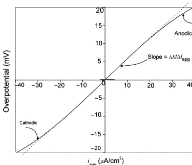
Figure 9 Current-potential relationships for a three-electrode system that shifts slightly (10-20 mV) from its equilibrium state [58]
