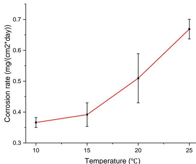
Figure 38 Corrosion rate of MC steel in 3.5 wt.% NaCl solution at different temperature
