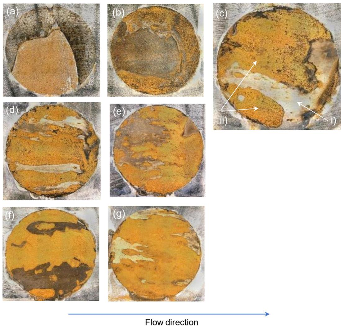
Figure 31 The evolution of the macro morphology of MC steel in NaCl solution with different flow velocity: (a) 0 rpm; (b) 50 rpm; (c) 100 rpm; (d) 200 rpm; (e) 300 rpm; (f) 400 rpm; (g) 500 rpm
