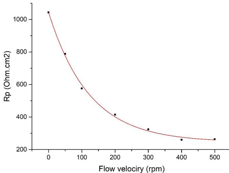
Figure 29 The evolution of final Rp at different flow velocities
