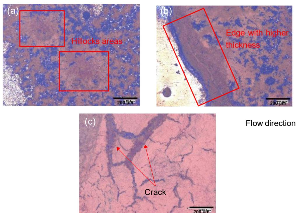
Figure 34 The morphology of rust layer of the sample with (a) 50 rpm; (b) 100 rpm; (c) 500 rpm flow velocity (water flows from bottom to top)
