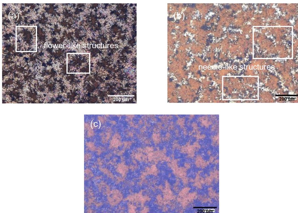
Figure 19 The morphology of rust layer of the sample immersed for (a) 1 day; (b) 4 days; (c) 7 days under  $\times 300$  magnification
