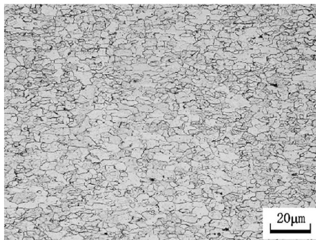
Figure 2 Metallographic microstructure of S420MC [17]
