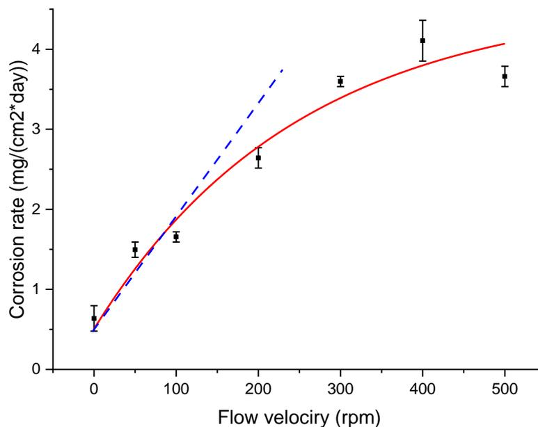
Figure 30 Corrosion rate of MC steel in 3.5 wt.% NaCl solution at different flow velocities
