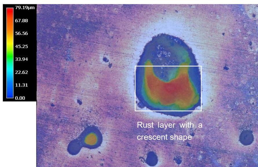
Figure A. 6 The height difference of microstructure of low-corrosion area of the sample with 100 rpm flow velocity
