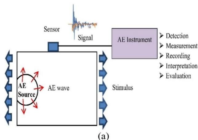
Figure 6 Schematic of AE monitoring freely rendered from [68]
