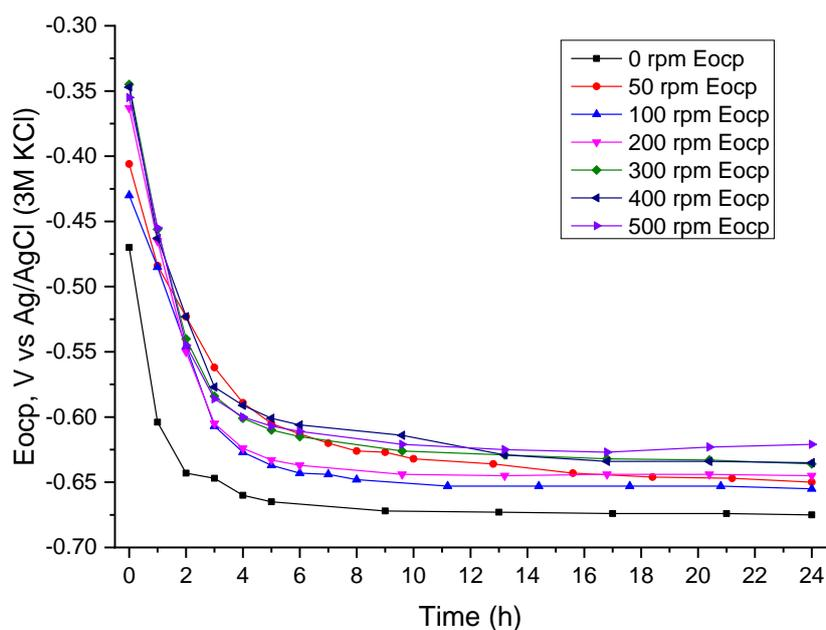
Figure 27 Evolutions of  $E_{OCP}$  of MC steel in 3.5 wt.% NaCl solution at different flow velocities
