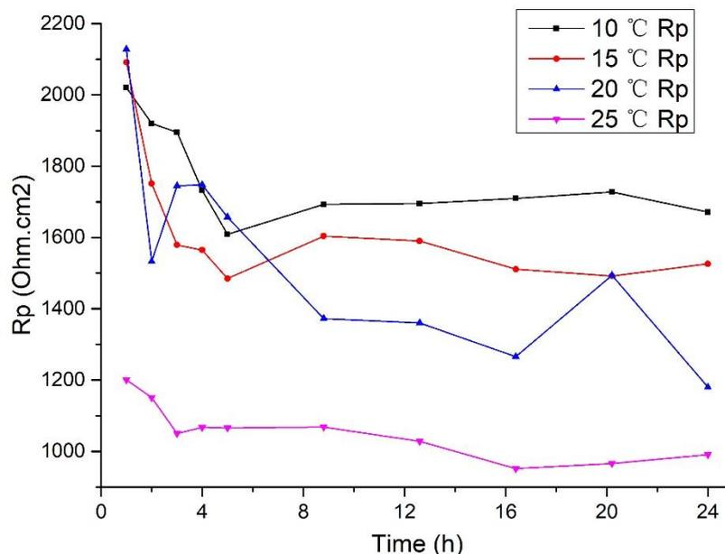
Figure 36 Time dependence of  $R_p$  for MC steel in 3.5 wt.% NaCl solution at different temperature
