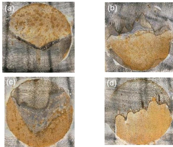
Figure 39 The evolution of the macro morphology of MC steel in NaCl solution with different temperatures: (a) 10 °C; (b) 15 °C; (c) 20 °C; (d) 25 °C
