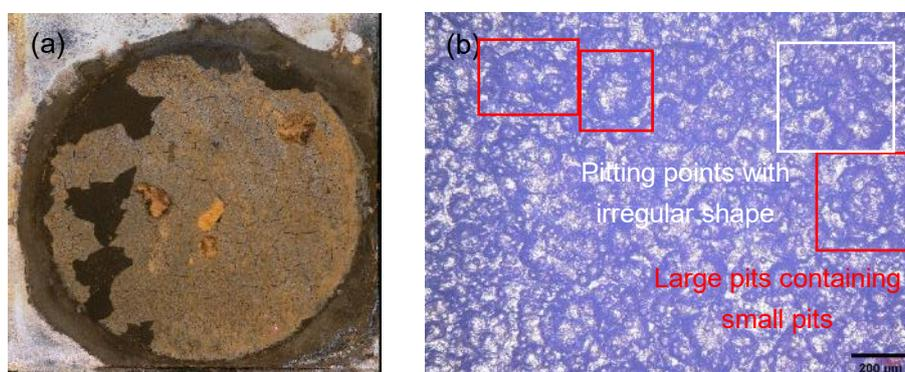
Figure 25 The morphology of MC steel in NaCl solution with OCP (a) macrostructure of rust layer; (b) microstructure at  $\times 200$  magnification without rust layer
