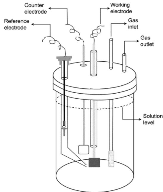
Figure 8 Three-electrode electrochemical cell for corrosion detection [58]
