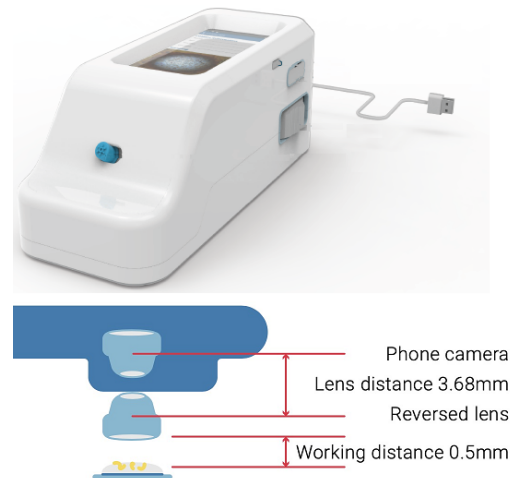
Fig. 4. Schistoscope SP (up) with working principle of sensor and lens combination (down)
