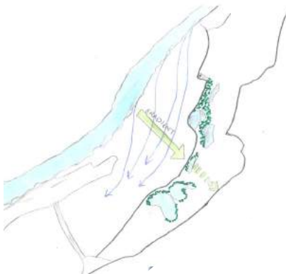
better flow of water with dike relocation
