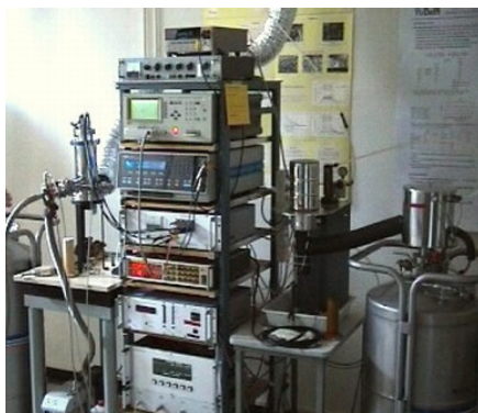
Fig. 7 Broadband Dielectric Spectroscopy set up.
