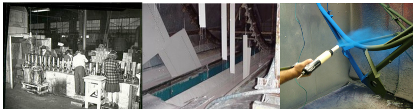
Fig. 1 Photo's of: an old fashioned (solvent) paint line (left); water borne paint line (middle); powder coating line (right).
