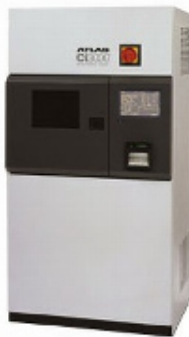
Fig. 5 Accelerated degradation technique: Weather-o-meter (WOM).
