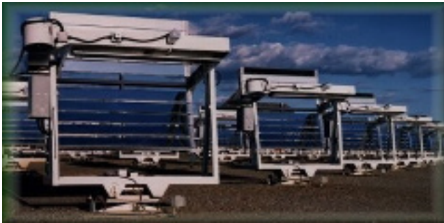
Fig. 4 Natural accelerated weathering in Florida, a Fresnel reflector.
