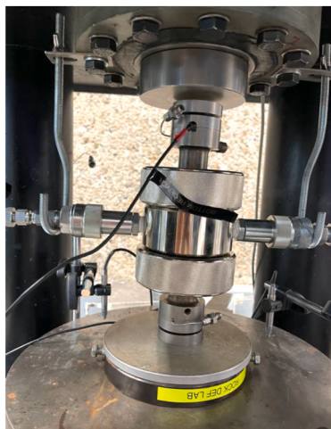
(c) Triaxial test setup
