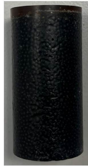
Fig. 12. SRR specimen after triaxial compression test at 20 MPa confining pressure.
