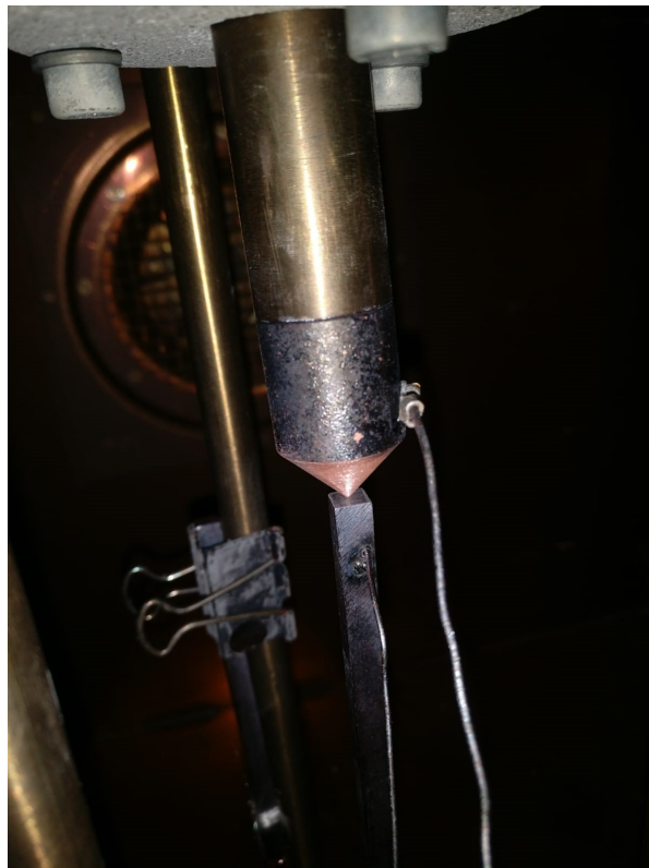
Figure B.5: Example of sanded contact point, this figure shows an sanded tip which is in contact with an sanded top surface of the sample.
