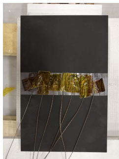
Figure 4.3: Thermocouple location (after experiment)
