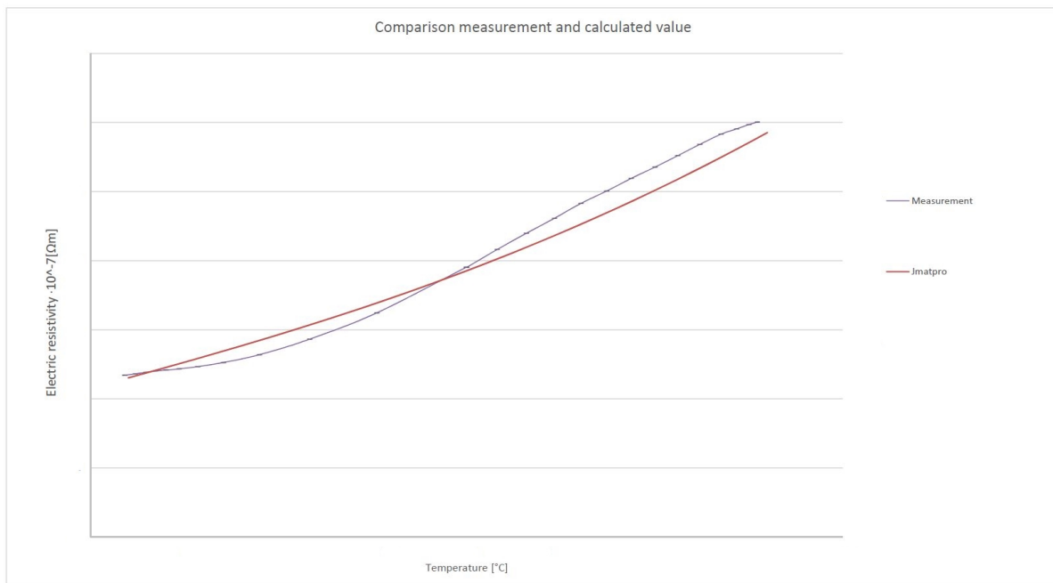
Figure 3.13: Comparison experimental measured data vs JMatPro, Electrical resistivity
