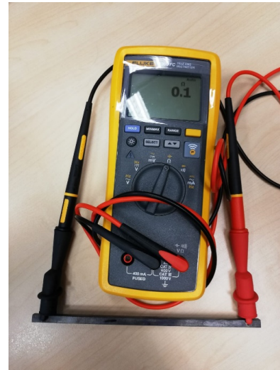
Figure 3.4: Resistance two point measurement on multimeter
