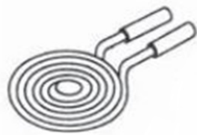
Figure 5.9: Pancake coil type, source [35]
