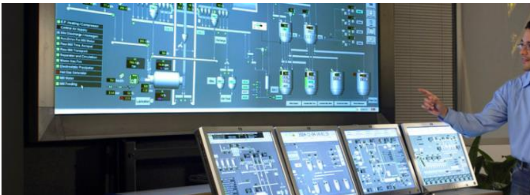
Figure 14. Human-machine interface for a SCADA system.
