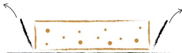
Figure 7: Opening the mold
