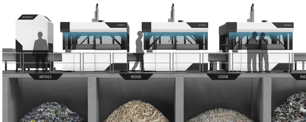
Fig. 3. ZenRobotics technology heavy picker sorting line [23]
