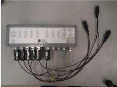
Figure 69 Conditioner box of the strain gauges
