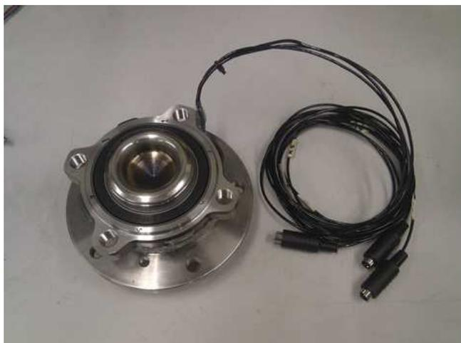
**Figure 1** A load sensing bearing
