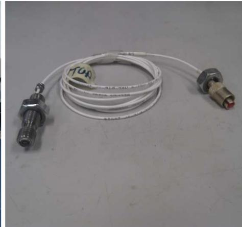
Figure 49 Eddy-current sensor
