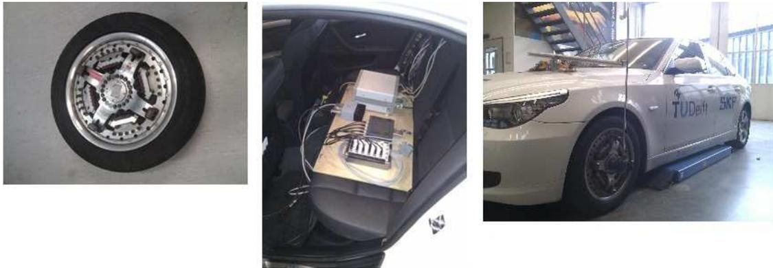
Figure 74 Left: VELOS wheel. Middle: Conditioning and power electronics. Right: VELOS mounted to the vehicle.
