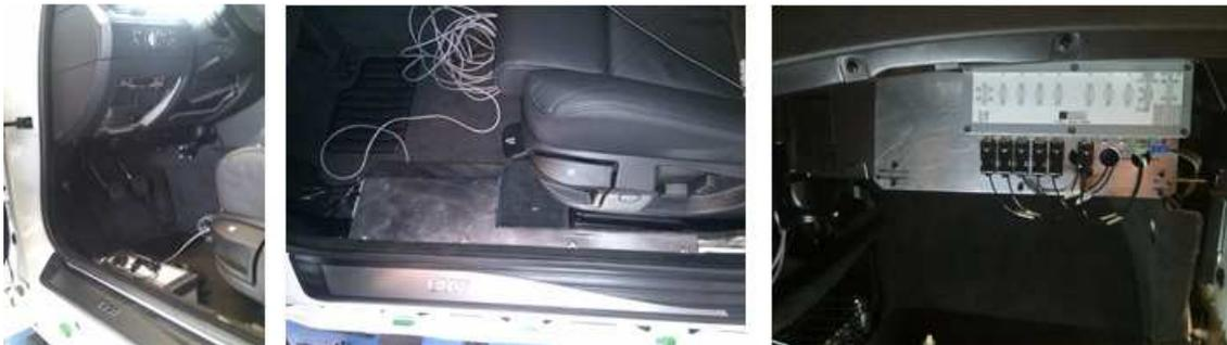
Figure 70 Conditioner box of the strain gauges installed in the vehicle
