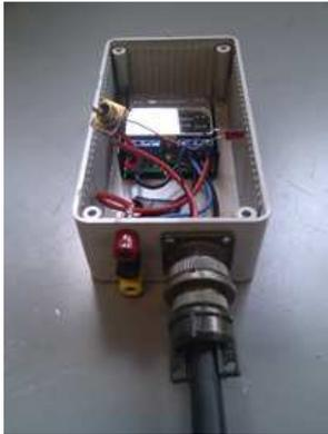
Figure 73 DC/DC-converter for the Eddy-current conditioner boxes
