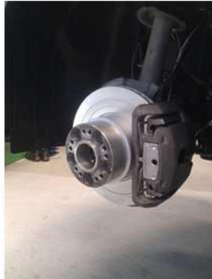
Figure 75 New brake disc and - calliper
