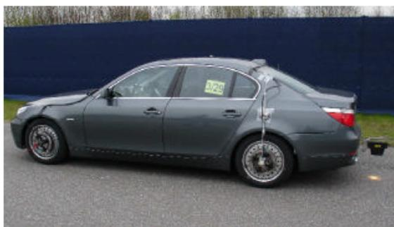
**Figure 11 MTS wheel force transducer assembly (Swift version)**
