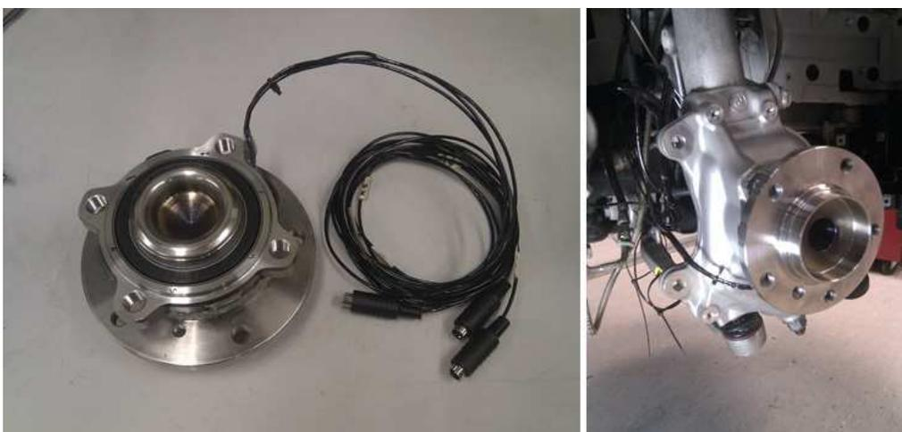
Figure 68 Load sensing bearing. Left: Single LSB. Right: Mounted in the vehicle.
