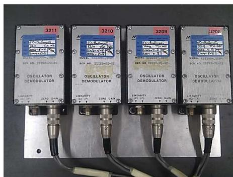
**Figure 51** Eddy-current signal conditioning electronics
