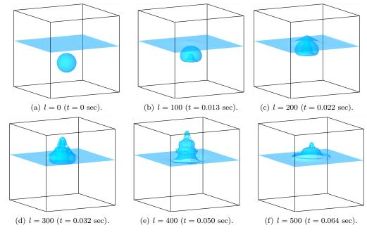
Fig. 2. Evolution of a rising bubble in water.
