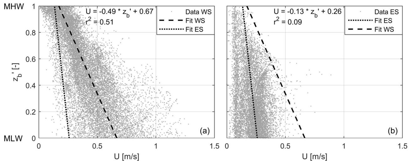
**Figure 6.** Bed level, scaled along mean low water (MLW; 0) and mean high water (MHW; 1), versus the average peak flow velocity from a 1 month simulation. All points on the intertidal areas of the full (a) Western Scheldt (WS) and (b) Eastern Scheldt (ES) are shown. Linear fits are provided with coefficients of determination ( $r^2$ ). The fits of both estuaries are shown in both graphs to allow comparisons.
