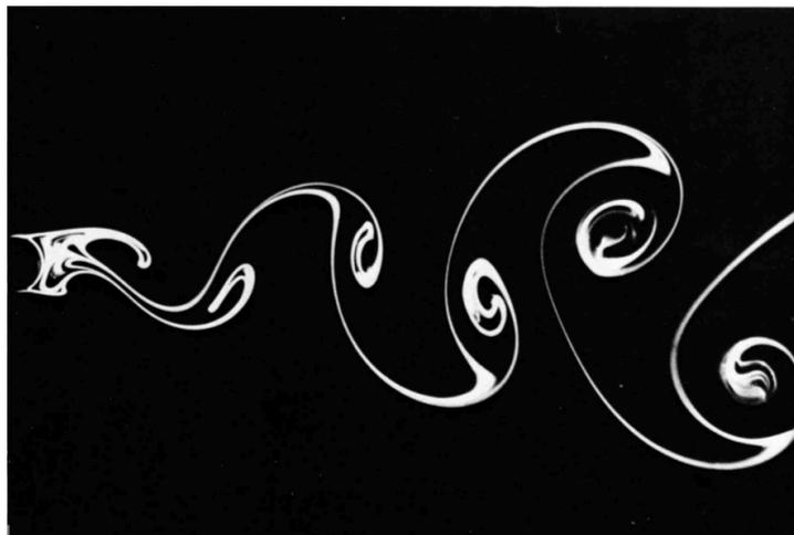
Figure 3.1: A Kármán vortex street behind a circular cylinder. This shows the complex wake structures that can occur in aerodynamic flow, which is an important consideration in unsteady aerodynamics [\[52\]](#).
