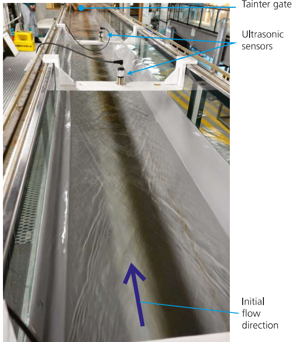
Figure 2. The experimental channel with Q=0.015 \text{ m}^3/\text{s} (looking downstream)
