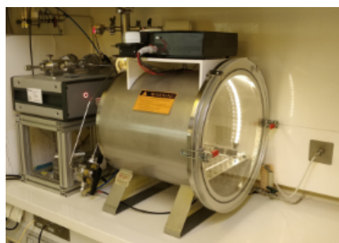
Fig. 2: Photograph of the nanomaterials printer (left) and a schematic diagram showing the major components and gas flow (right)
