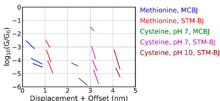
**Figure 5.** Comparison of the average conductance plateaus for methionine and cysteine obtained from the clustering analysis into 5 classes as measured by the two break-junction techniques. Plateaus (slanted line segments) are only shown if they are shorter than the amino acid and less steep than the tunneling slope. The plateau positions for subsequent molecules are offset by 1 nm in the horizontal displacement axis. The MCBJ data are the same as in Figure 4.
