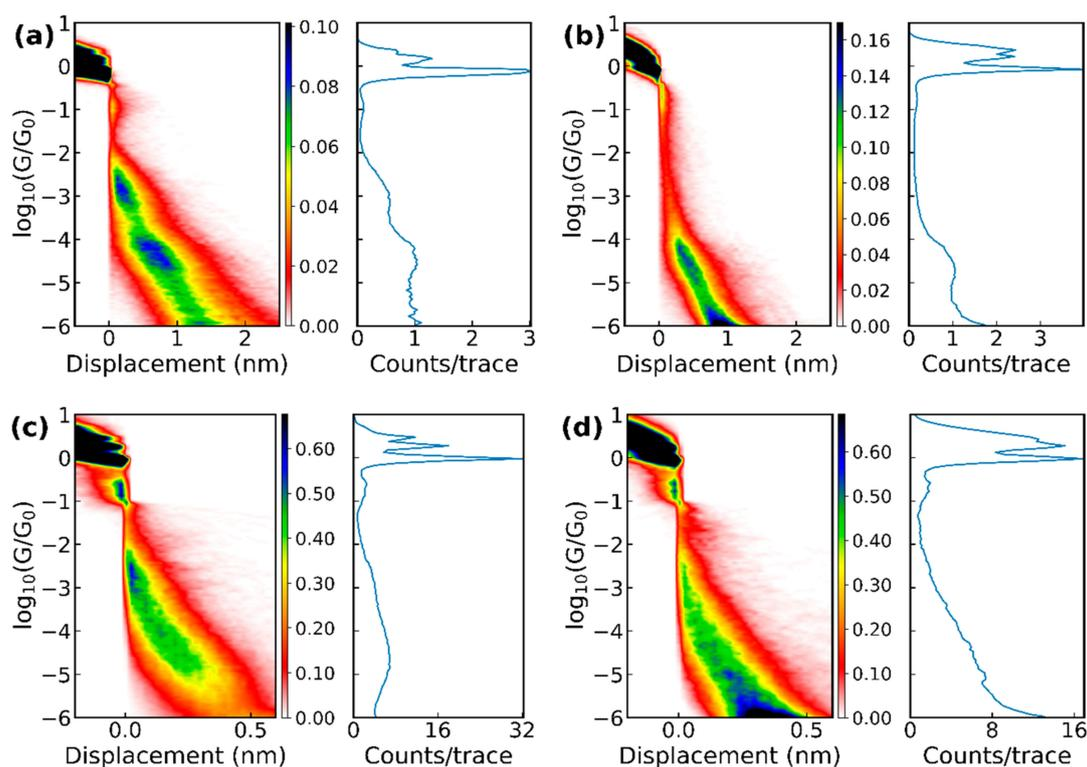
**Figure 3.** 1D and 2D histograms of the raw data of (a) 6000 breaking traces of methionine and (b) 4000 breaking traces of cysteine measured with the MCBJ setup, as well as (c) 5745 traces of methionine and (d) 3584 traces of cysteine at pH = 7 measured with the STM-BJ.
