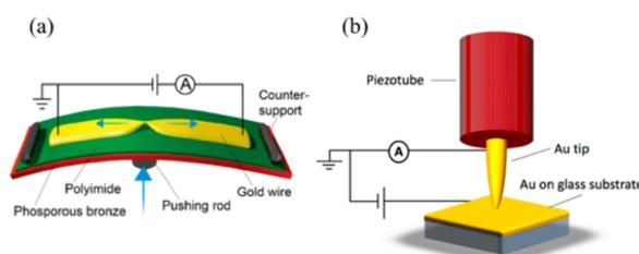
**Figure 2.** (a) Sketch of the mechanically controlled break junction MCBJ setup (from Reference [23]). The sample is bent and consequently broken by moving the pushing rod up; (b) schematic representation of the scanning tunneling microscopy break-junction (STM-BJ) setup. The motion of the tip is controlled by the piezotube [20].
